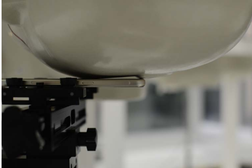
SAR Test Setup Photo 3 – Left Cheek
