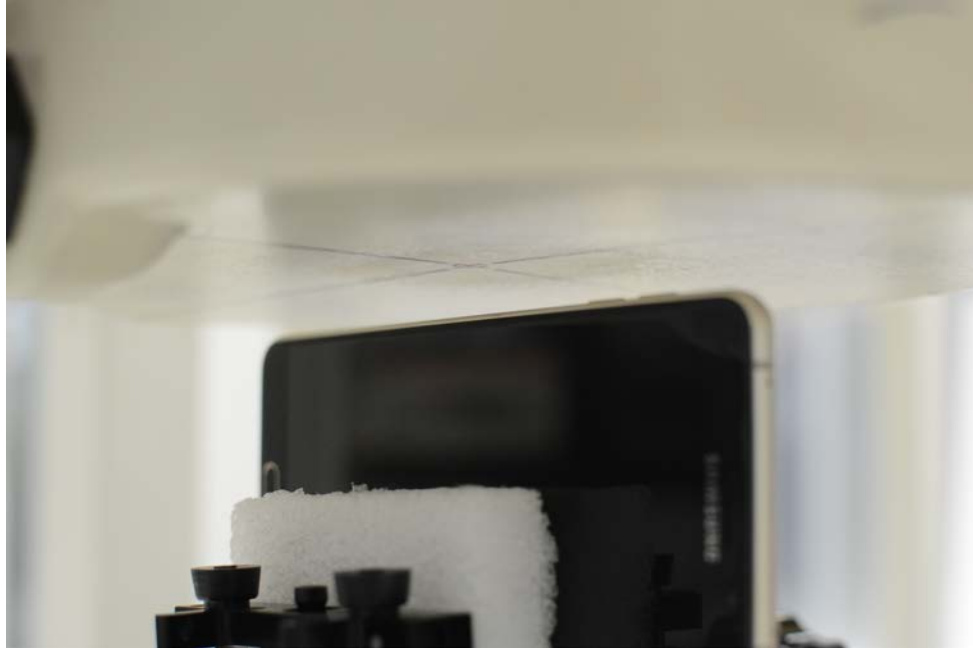
SAR Test Setup Photo 13 – Left Edge (10 mm)
