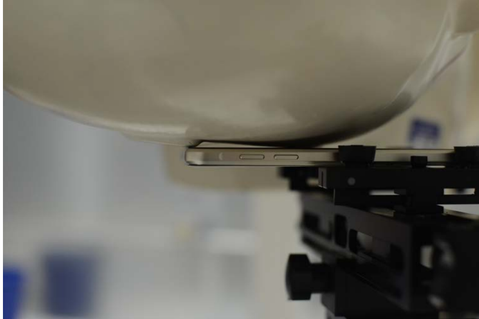
SAR Test Setup Photo 1 –Right Cheek
