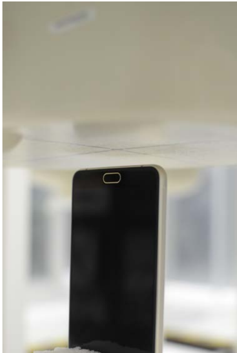
SAR Test Setup Photo 11 – Bottom Edge (10 mm)
