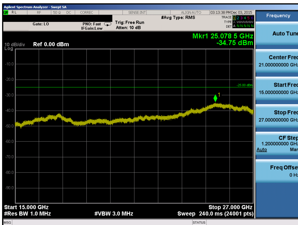
Plot 7-34. Conducted Spurious Plot (Band 41 – 5.0MHz QPSK – RB Size 1, RB Offset 0 – High Channel)
