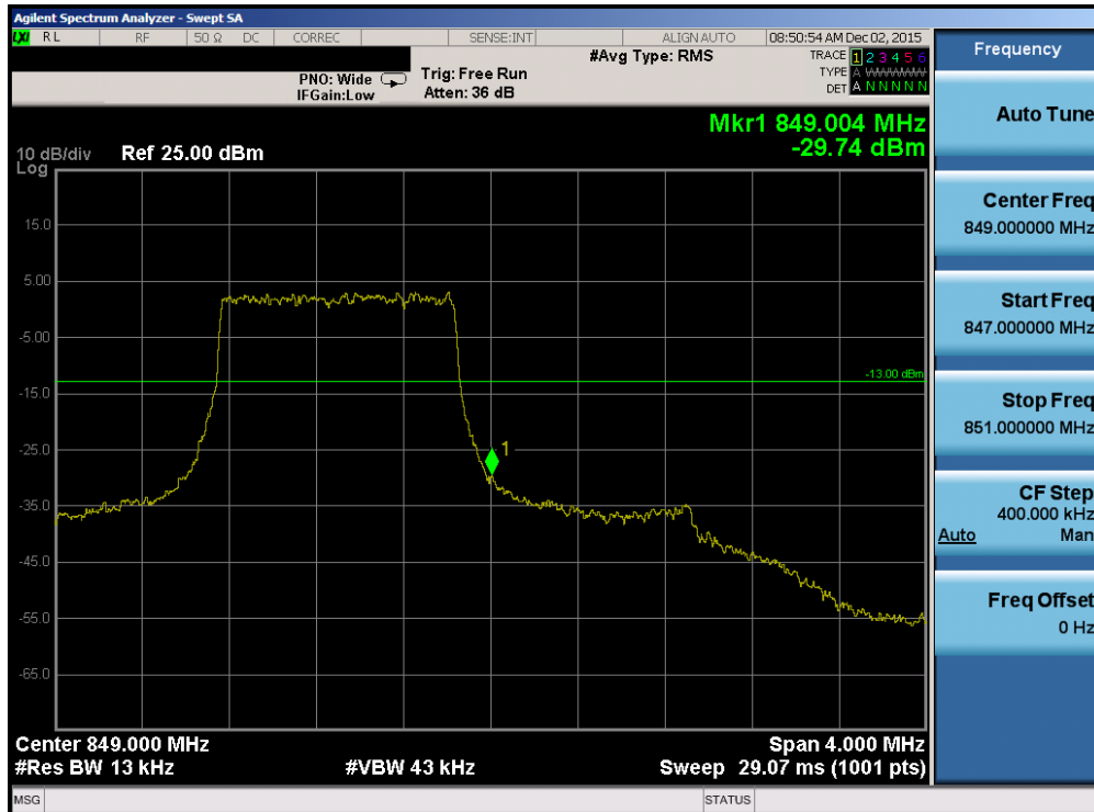
Plot 7-37. Upper Band Edge Plot (Band 5 – 1.4MHz QPSK – RB Size 6)
