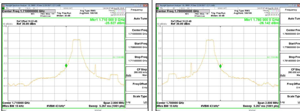
LTE B66 1.4MHz QPSK Low Channel RB1-0
