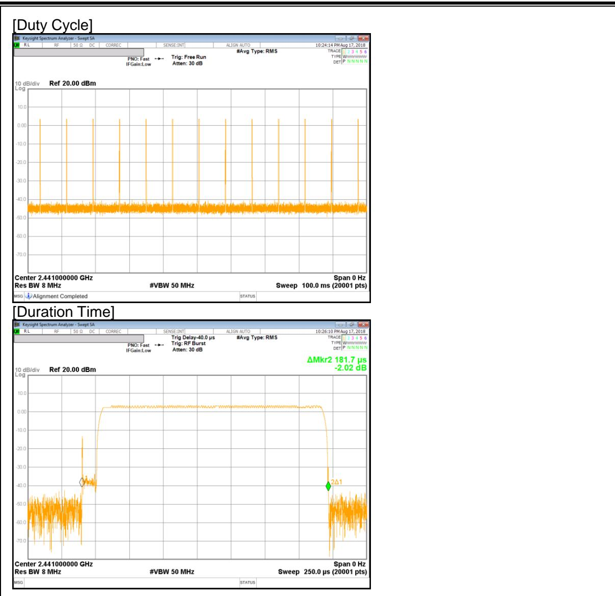
**Duty Cycle Factor =  $20\log(\text{number of signal} \times \text{Transmission time} / 100)$**
