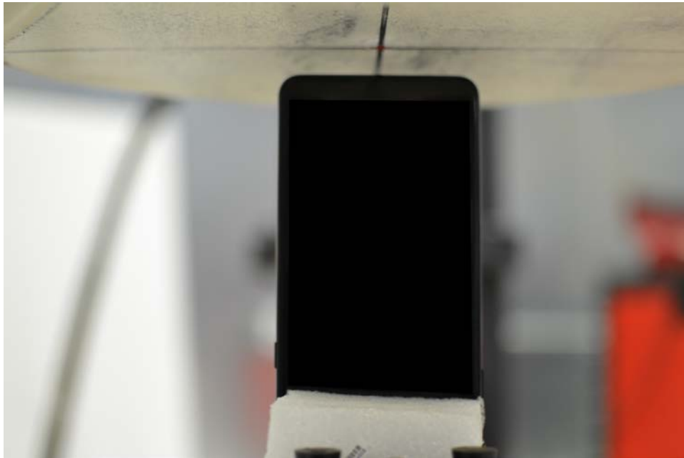
SAR Test Setup Photo 8: Bottom at 1.0 cm
