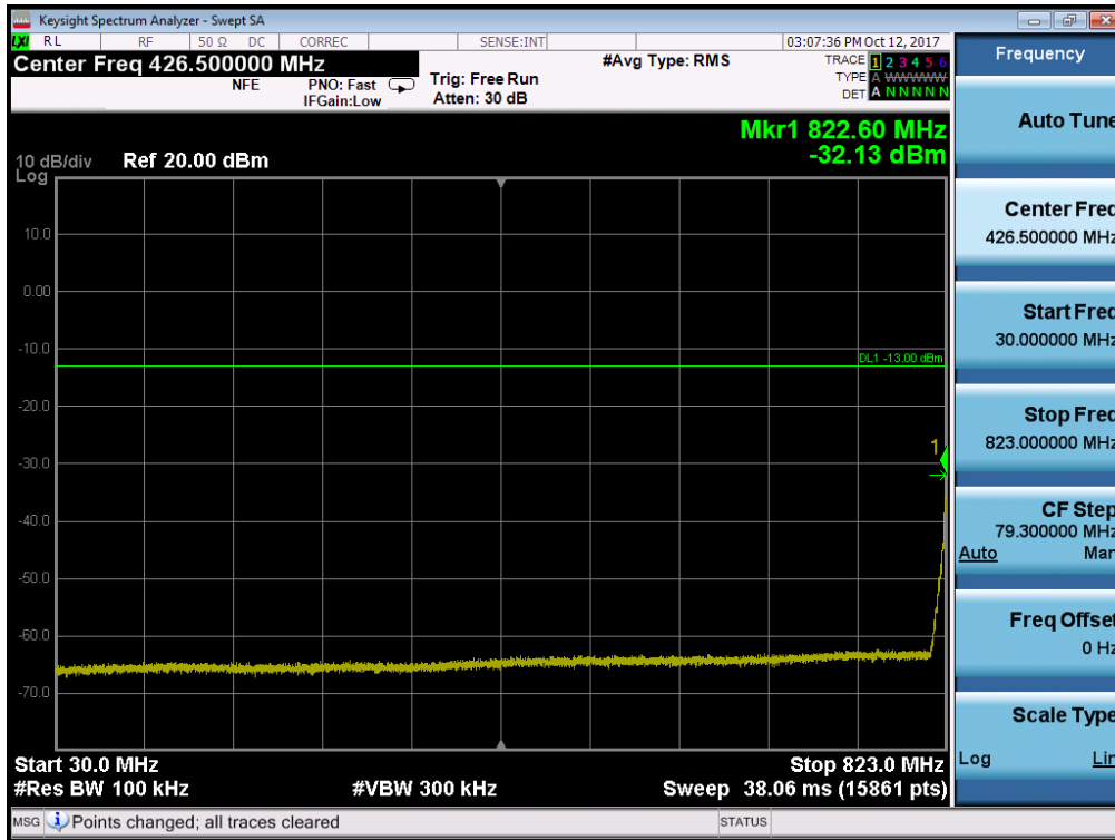
Plot 7-26. Conducted Spurious Plot (Cellular WCDMA Mode - Low Channel)
