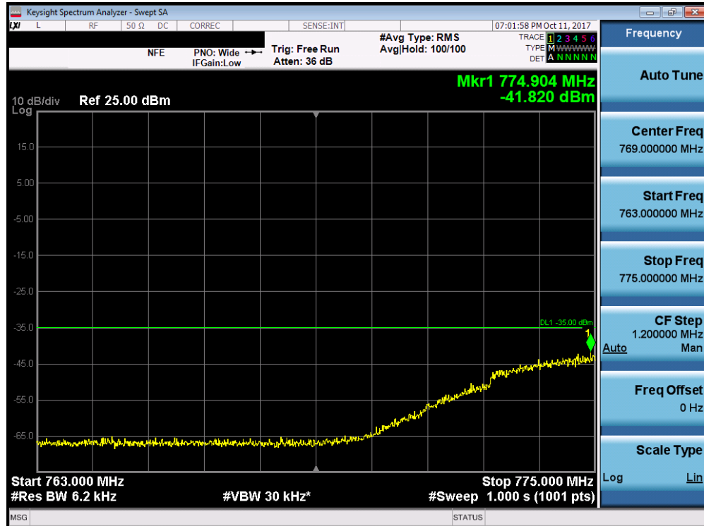
Plot 7-143. Lower Emission Mask Edge Plot (Band 13 - 5.0MHz QPSK - Full RB Configuration)
