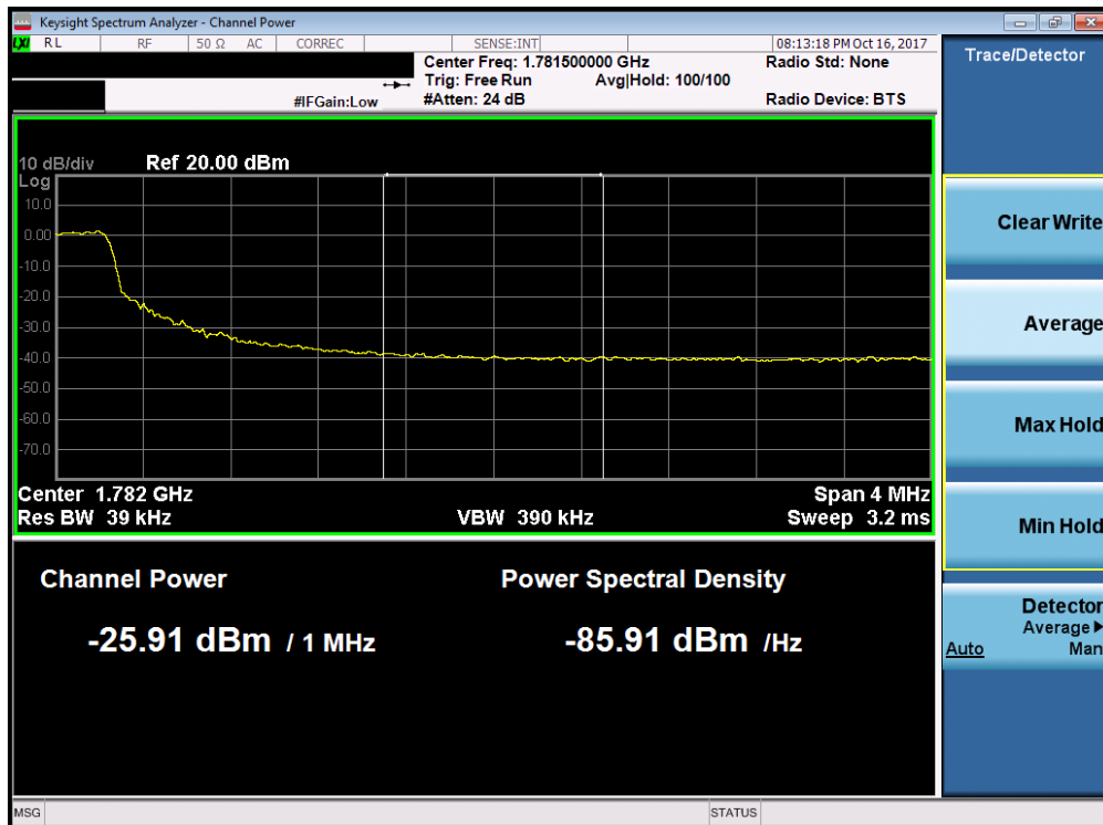
Plot 7-177. . Upper Extended Band Edge Plot (Band 66 - 5.0MHz QPSK - Full RB Configuration)
