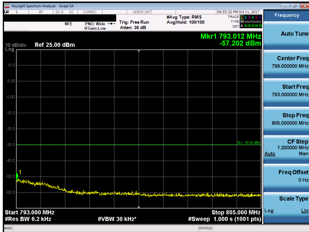
Plot 7-145. Upper Emission Mask Edge Plot (Band 13 - 5.0MHz QPSK - Full RB Configuration)
