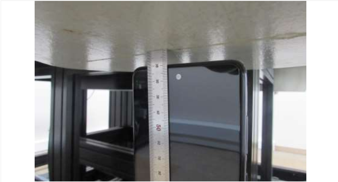
Distance of 10 mm from the EUT
