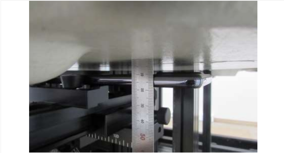
Distance of 10 mm from the EUT
