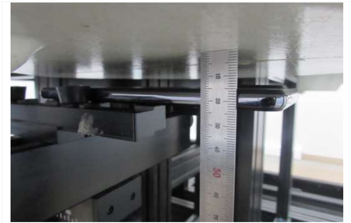
Distance of 15 mm from the EUT
