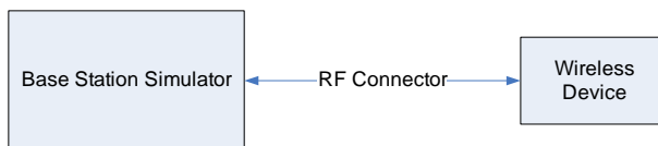
Figure 9-2 Power Measurement Setup
