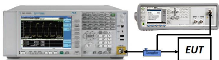
Figure 7-5. Test Instrument & Measurement Setup
