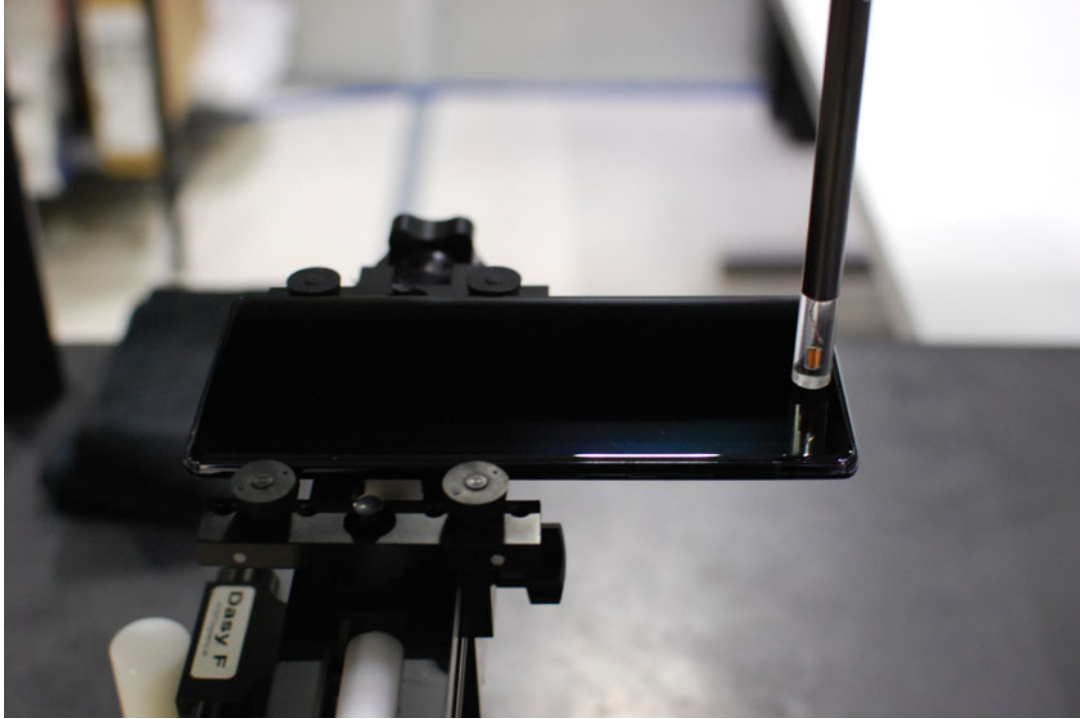
Figure 16-1 Test Setup for Wireless Device
