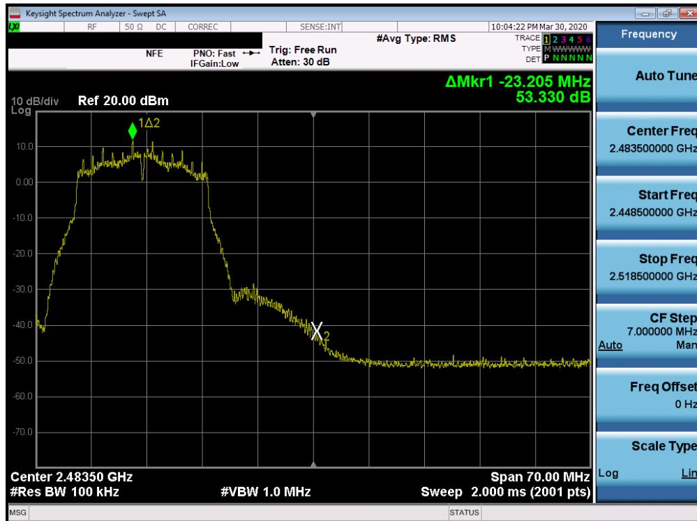
Plot 7-22. Band Edge Plot (802.11g – Ch. 11)
