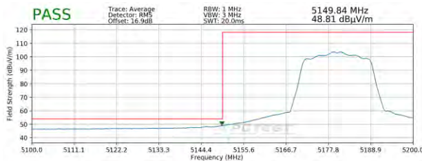
Plot 7-85. Radiated Lower Band Edge Plot (Average – UNII Band 1)
