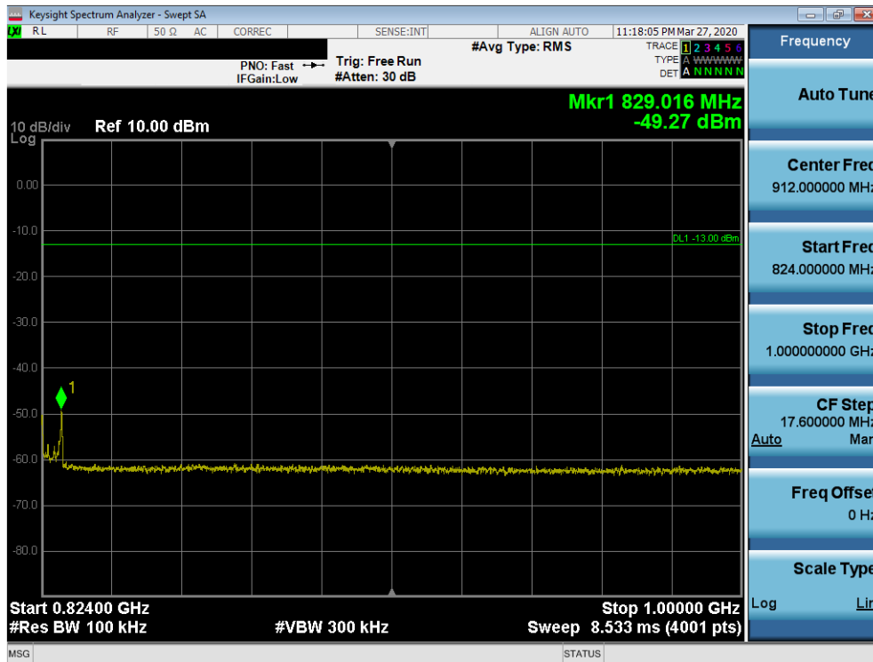
Plot 7-31. Conducted Spurious Plot (LTE Band 26 - 15MHz QPSK - RB Size 1, RB Offset 0)
