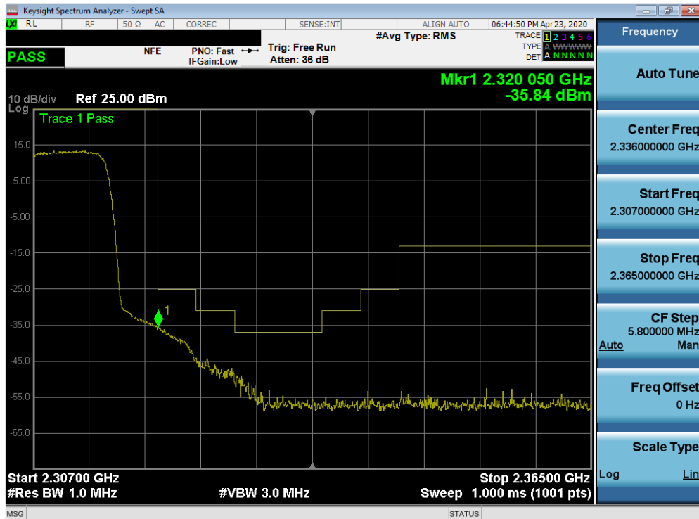
Plot 7-532. Upper Extended Band Edge Plot (Band 30 - 10.0MHz QPSK - Full RB Configuration)
