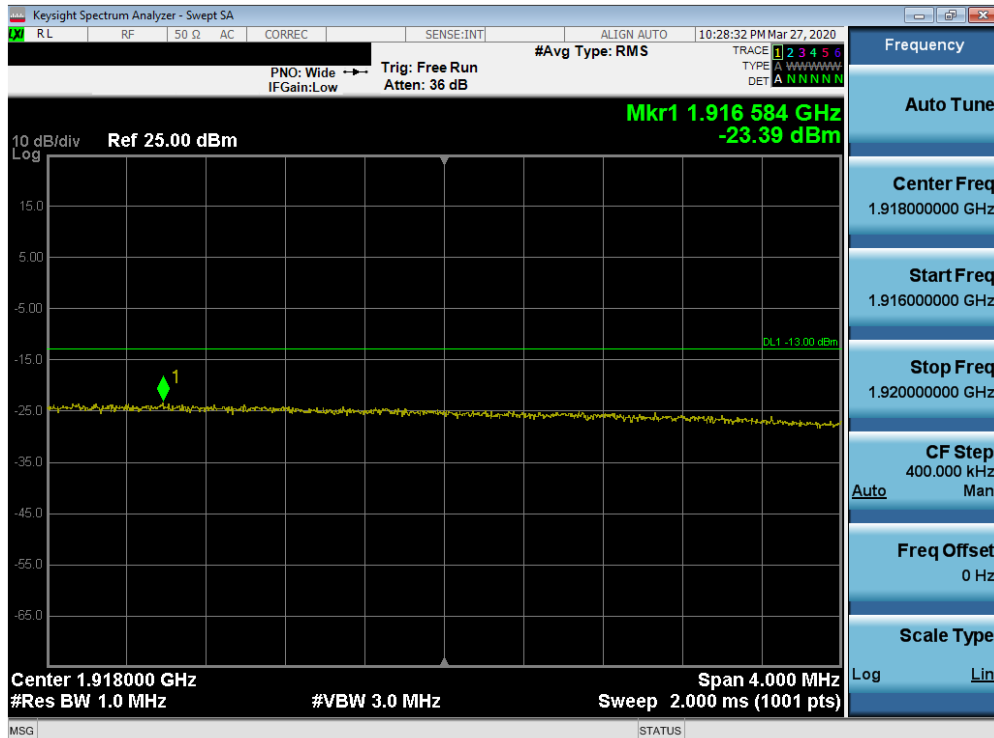
Plot 7-502. Upper Extended Band Edge Plot (Band 25 - 15.0MHz QPSK - Full RB Configuration)
