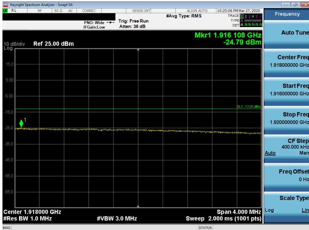
Plot 7-508. Upper Extended Band Edge Plot (Band 25 - 20.0MHz QPSK - Full RB Configuration)
