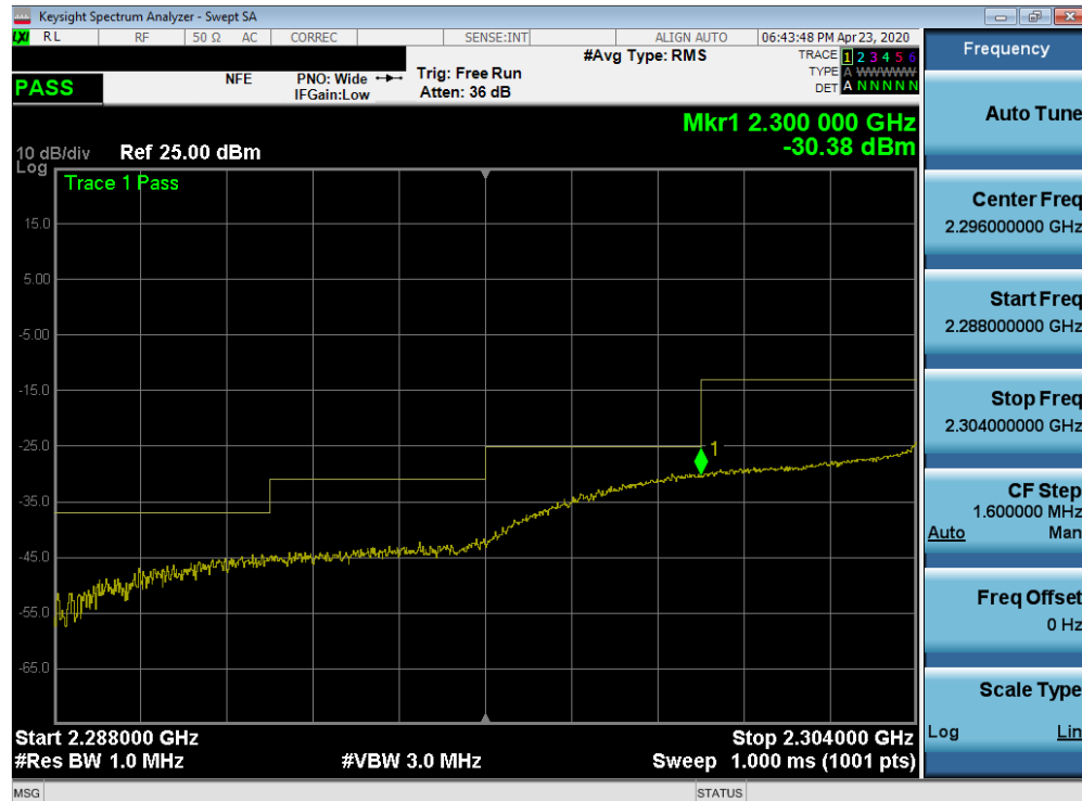
Plot 7-530. Lower Extended Band Edge Plot (Band 30 - 10.0MHz QPSK - Full RB Configuration)
