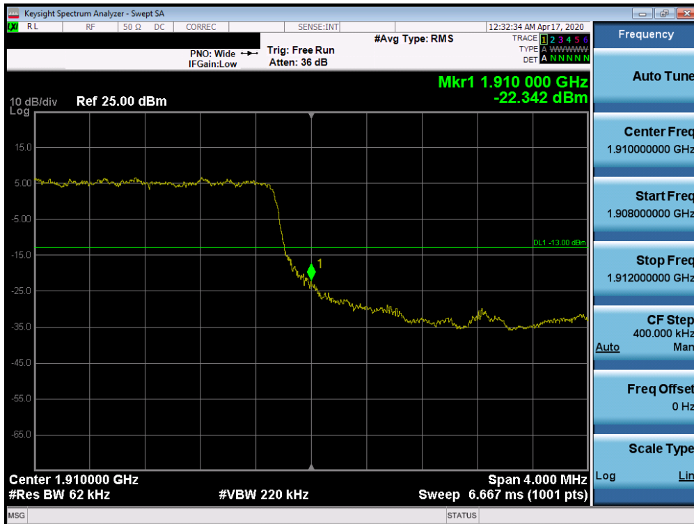
Plot 7-512. Upper Extended Band Edge Plot (n2 - 5MHz DFT-s-OFDM-QPSK - Full RB Configuration)
