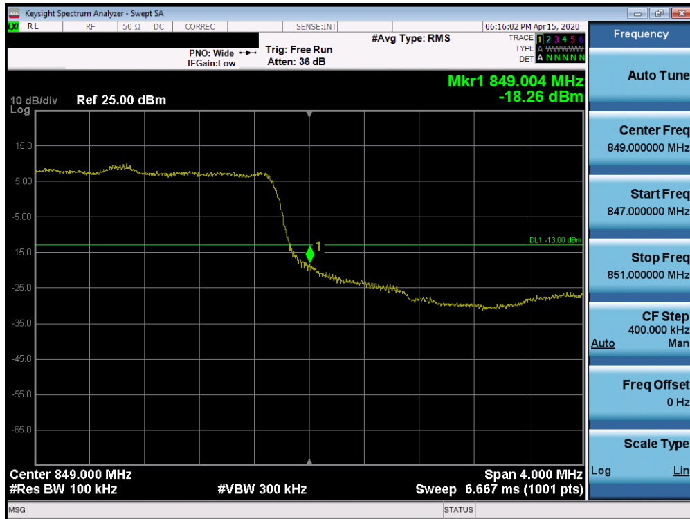
Plot 7-414. Upper Band Edge Plot (n5 – 5.0MHz DFT-s-OFDM BPSK - Full RB Configuration)
