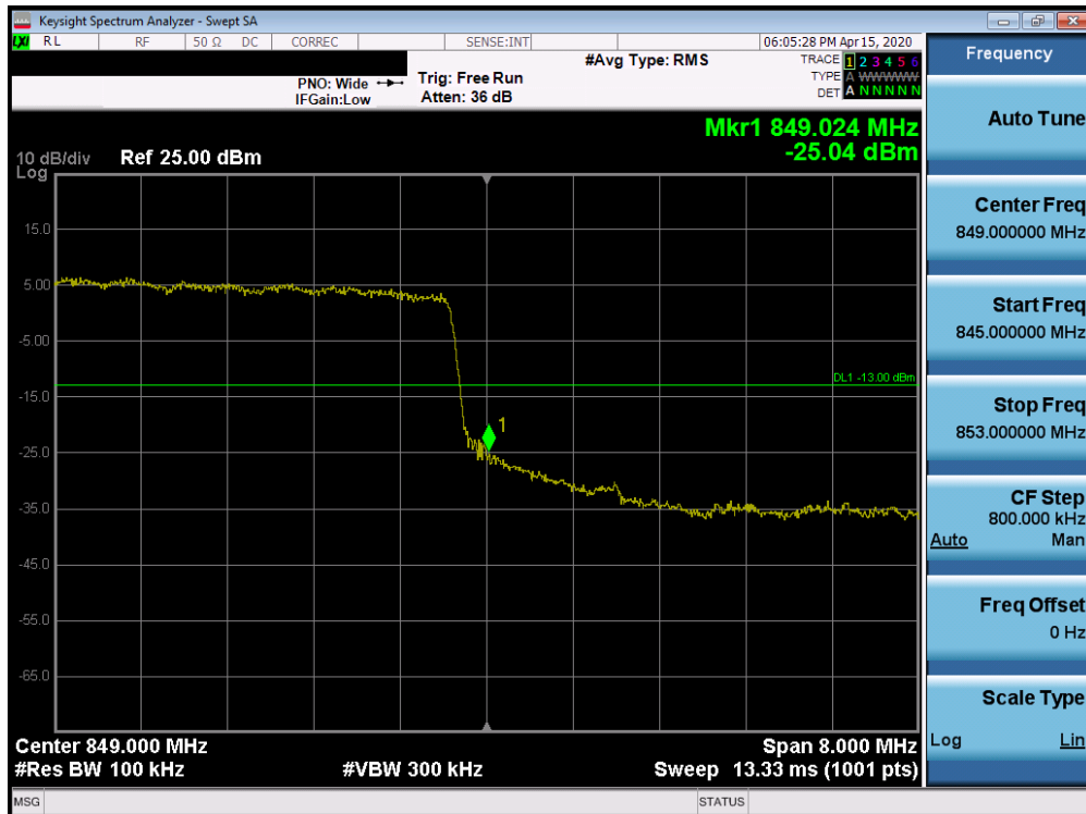
Plot 7-416. Upper Band Edge Plot (n5 – 10.0MHz DFT-s-OFDM BPSK - Full RB Configuration)
