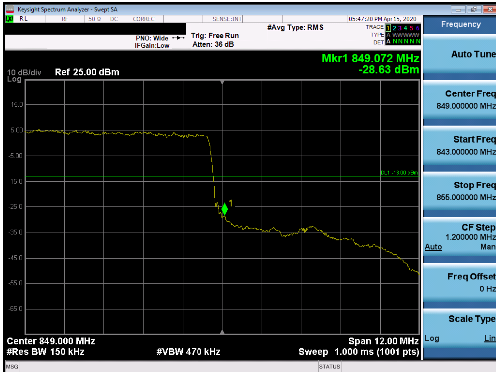
Plot 7-418. Upper Band Edge Plot (n5 – 15.0MHz DFT-s-OFDM BPSK - Full RB Configuration)
