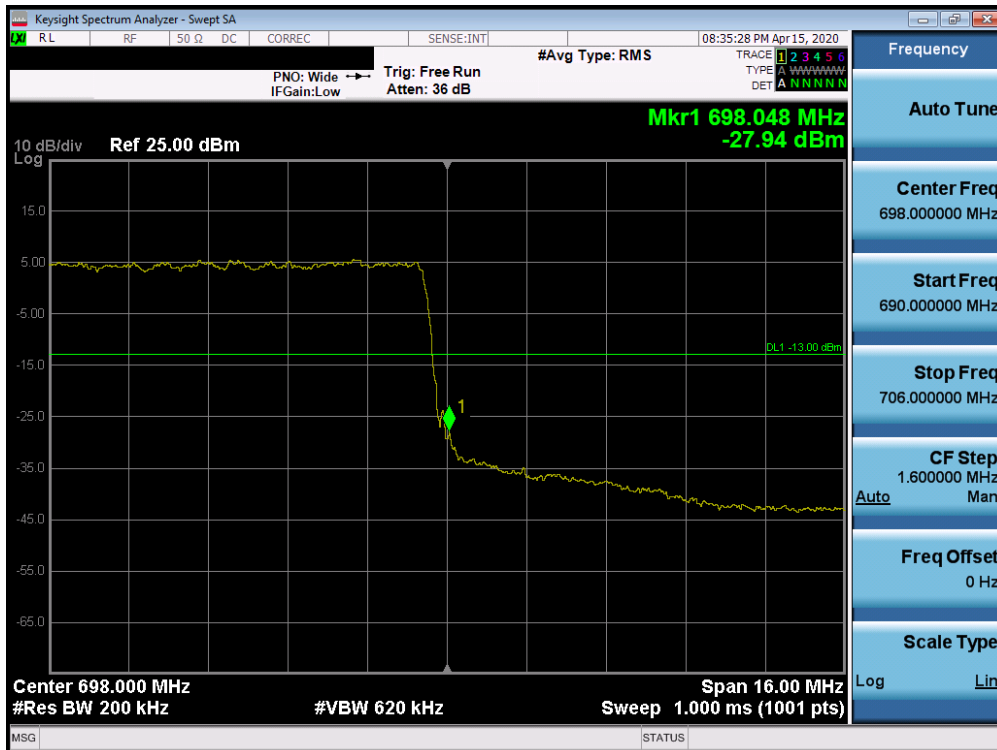
Plot 7-390. Upper Band Edge Plot (n71 - 20MHz DFT-s -OFDM-QPSK - Full RB Configuration)
