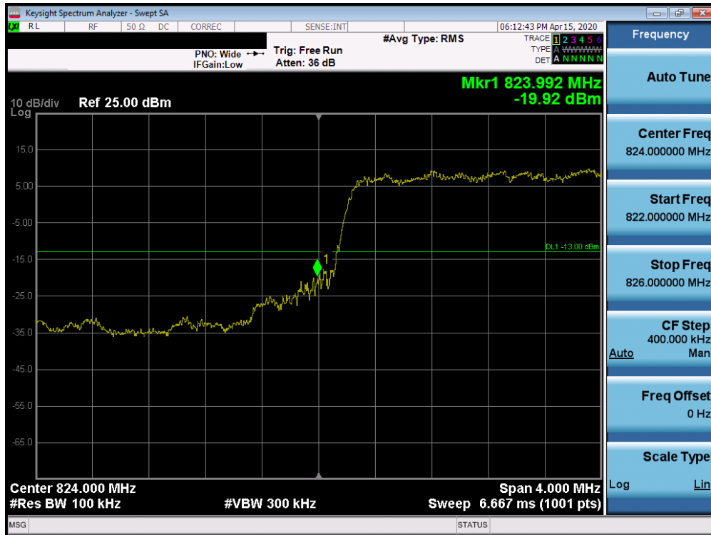
Plot 7-413. Lower Band Edge Plot (n5 – 5.0MHz DFT-s-OFDM BPSK - Full RB Configuration)
