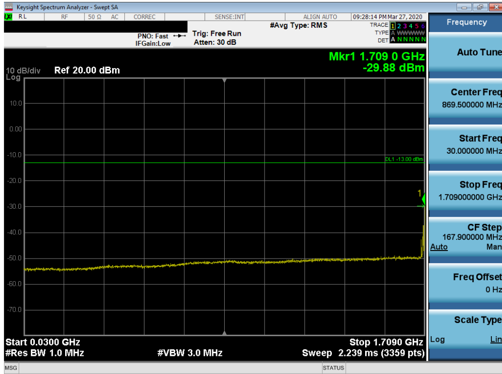
Plot 7-296. Conducted Spurious Plot (Band 66/4 - 20.0MHz QPSK - RB Size 1, RB Offset 0 - Low Channel)
