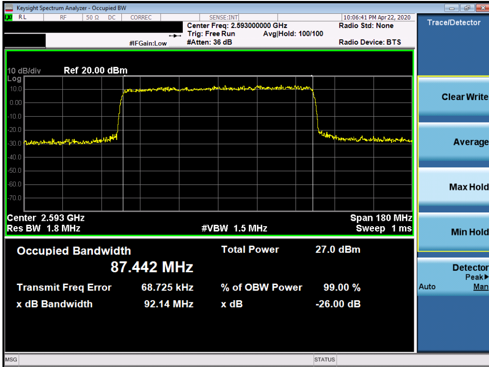
Plot 7-232. Occupied Bandwidth Plot (n41 90MHz 64QAM-CP-OFDM- Full RB Configuration)
