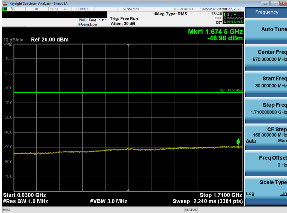
Plot 7-302. Conducted Spurious Plot (Band 66/4 - 20.0MHz QPSK - RB Size 1, RB Offset 0 - High Channel)
