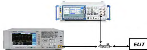
Figure 7-2. Test Instrument & Measurement Setup
