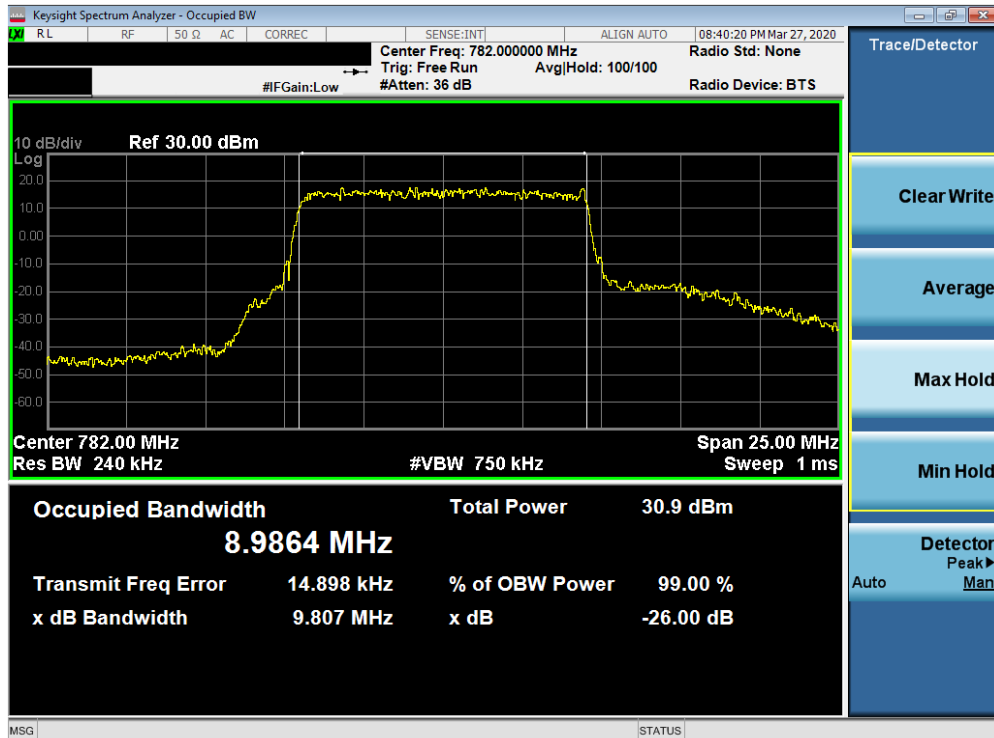
Plot 7-48. Occupied Bandwidth Plot (Band 13 - 10.0MHz QPSK - Full RB Configuration)
