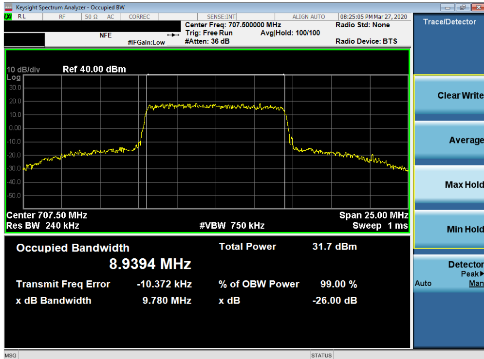
Plot 7-42. Occupied Bandwidth Plot (Band 12 - 10.0MHz QPSK - Full RB Configuration)
