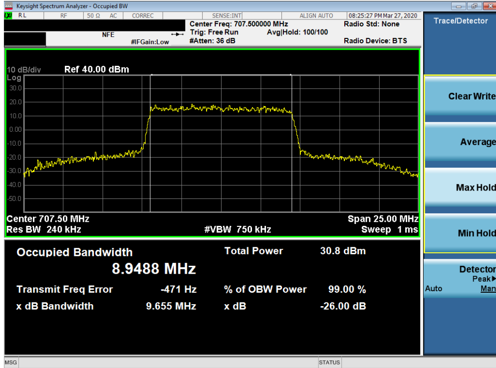
Plot 7-43. Occupied Bandwidth Plot (Band 12 - 10.0MHz 16-QAM - Full RB Configuration)
