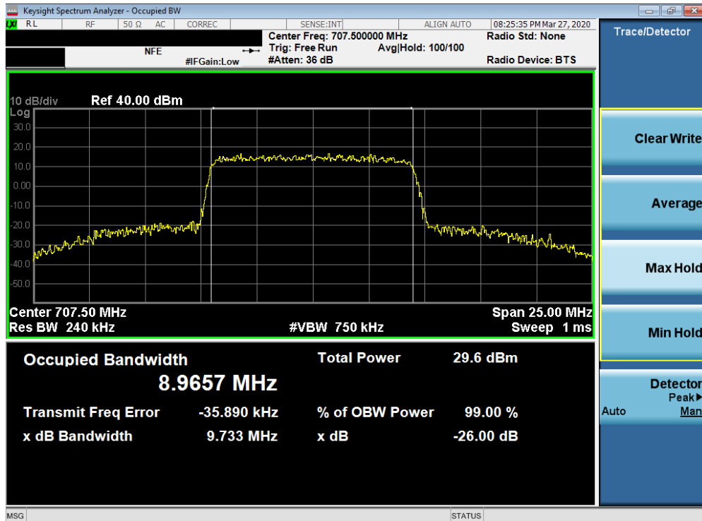
Plot 7-44. Occupied Bandwidth Plot (Band 12 - 10.0MHz 64-QAM - Full RB Configuration)
