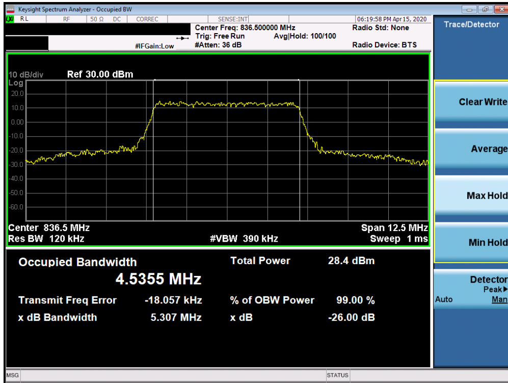
Plot 7-67. Occupied Bandwidth Plot (n5 5MHz QPSK-CP-OFDM - Full RB Configuration)
