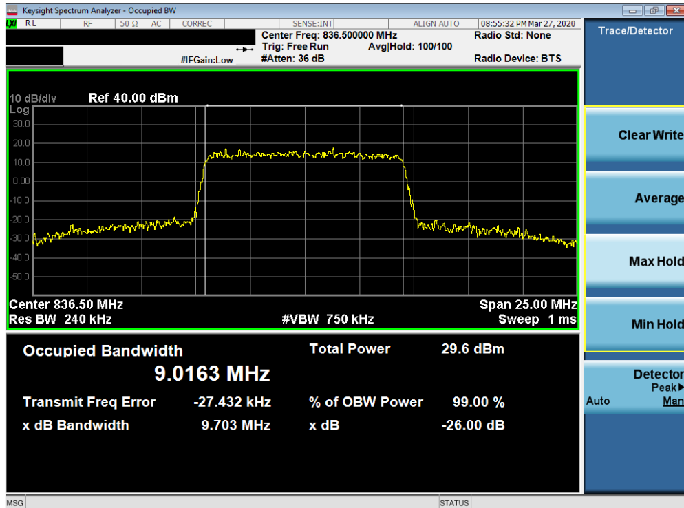
Plot 7-62. Occupied Bandwidth Plot (Band 26/5 - 10.0MHz 64-QAM - Full RB Configuration)
