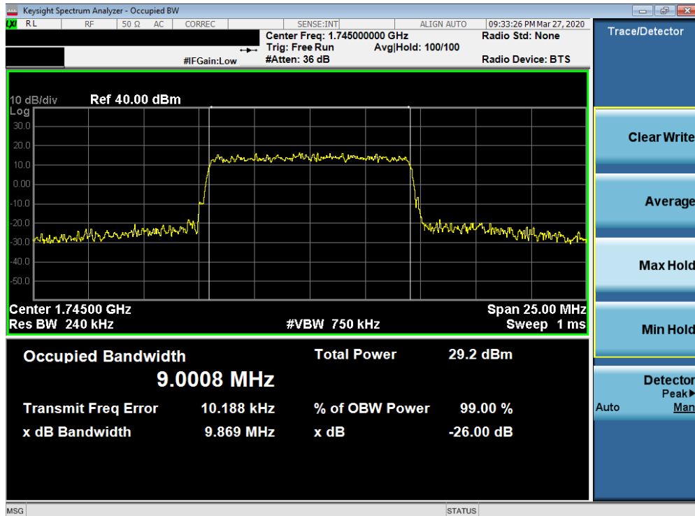
Plot 7-97. Occupied Bandwidth Plot (Band 66/4 - 10.0MHz 64-QAM - Full RB Configuration)
