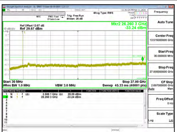
LTE B41 10MHz 16QAM Middle Channel RB1-0
