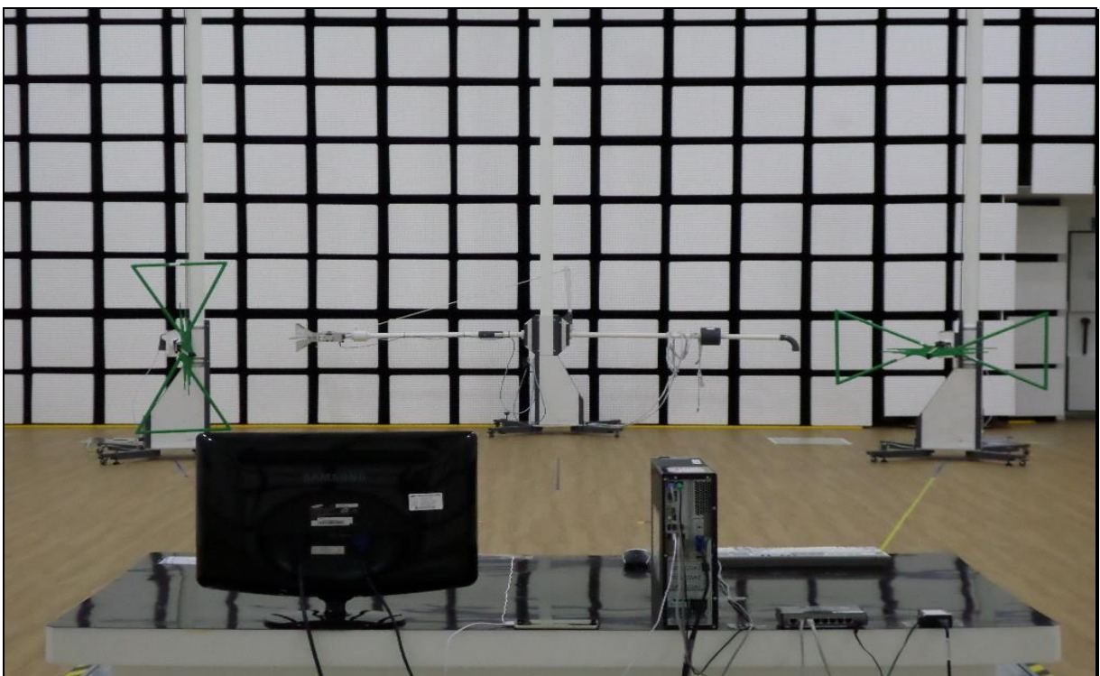
[ Radiated Disturbance for Below 1 GHz – Rear ]
