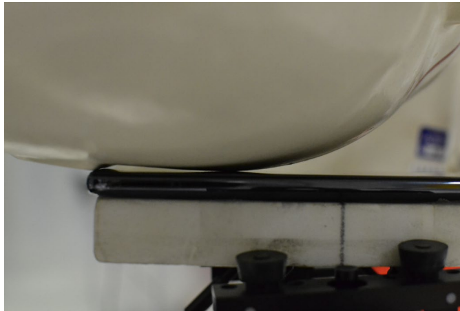
SAR Test Setup Photo 1 – Right Cheek
