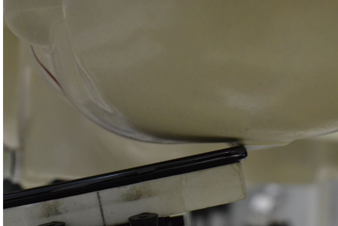
SAR Test Setup Photo 4 – Left Tilt
