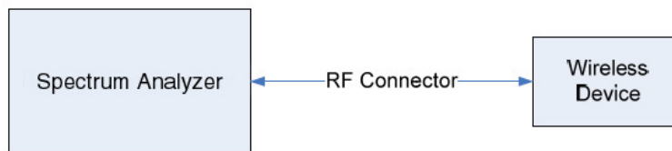
Figure 7-1. Test Instrument & Measurement Setup
