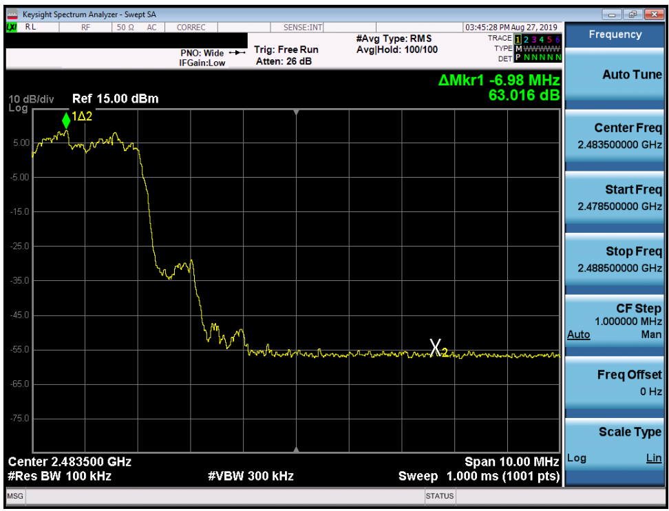
Plot 7-31. Band Edge Plot (Bluetooth with Hopping Enabled, 3 Mbps)
