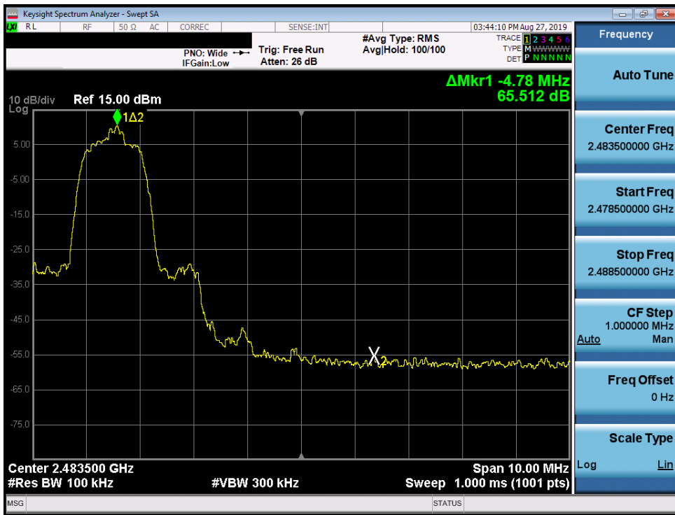
Plot 7-29. Band Edge Plot (Bluetooth with Hopping Disabled, 3 Mbps – Ch. 78)
