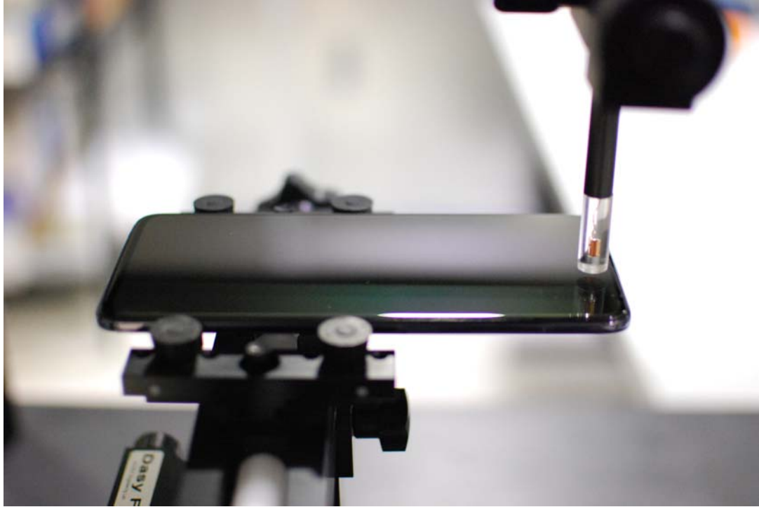
Figure 16-1 Test Setup for Wireless Device
