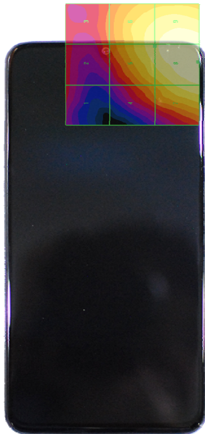
Figure 17-4 E-Field WD Scan overlay (T-Coil Centered scan area pictured)
