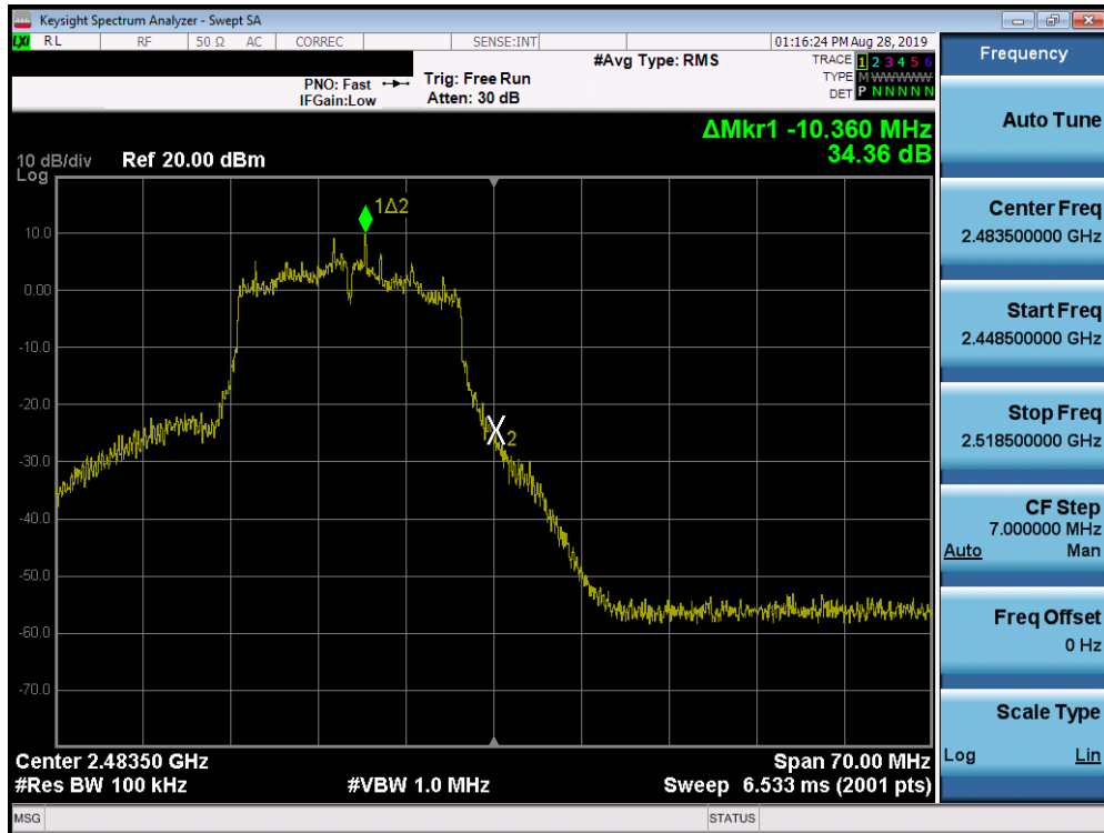
Plot 7-30. Band Edge Plot (802.11n (2.4GHz) – Ch. 13)
