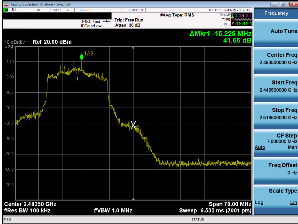
Plot 7-29. Band Edge Plot (802.11n (2.4GHz) – Ch. 12)
