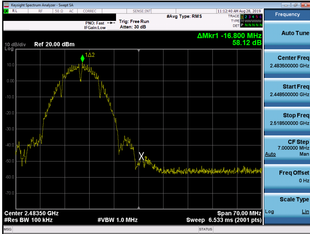
Plot 7-21. Band Edge Plot (802.11b – Ch. 12)
