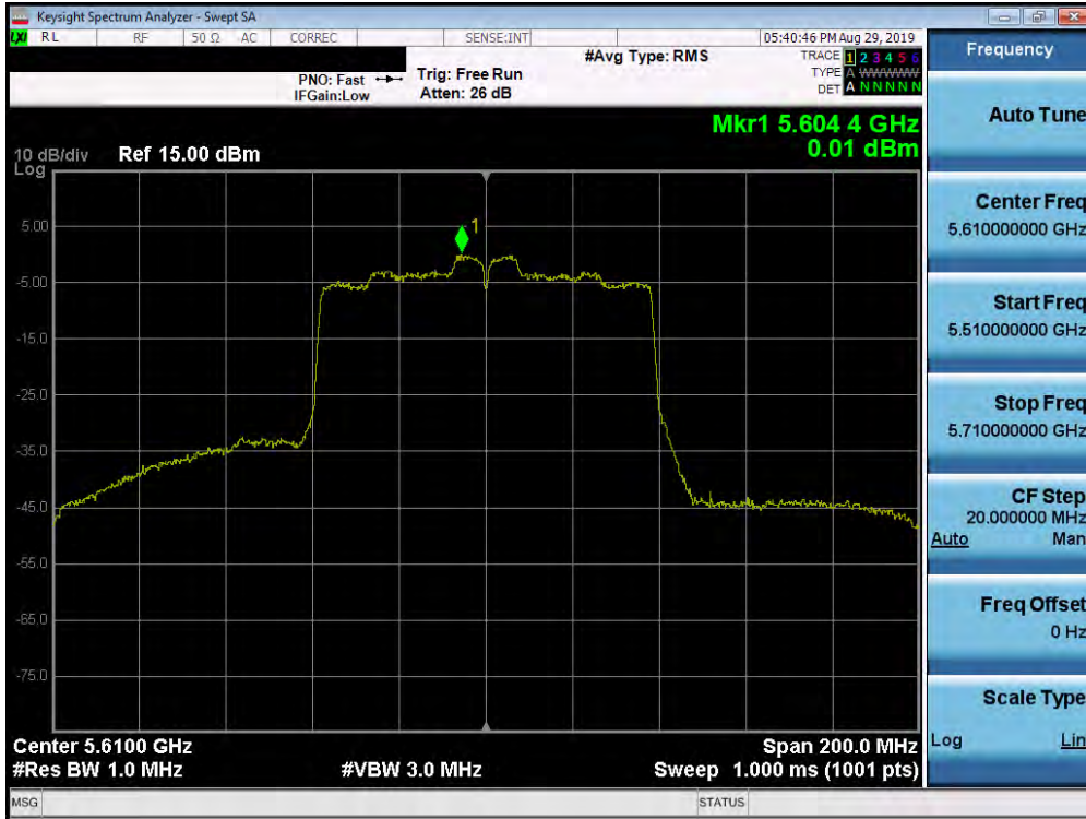
Plot 7-68. Power Spectral Density Plot (80MHz BW 802.11ac (UNII Band 2C) – Ch. 122)
