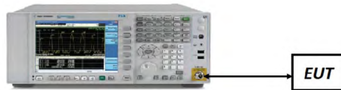
Figure 7-4. Test Instrument & Measurement Setup
