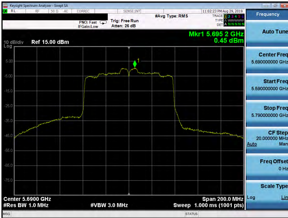
Plot 7-69. Power Spectral Density Plot (80MHz BW 802.11ac (UNII Band 2C) – Ch. 138)
