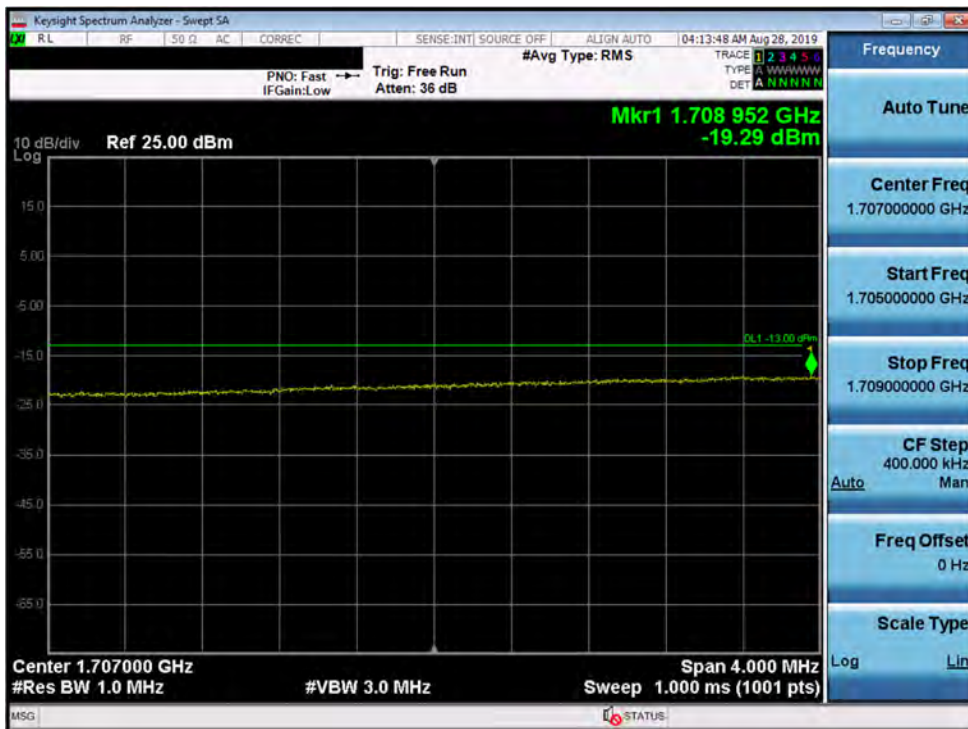
Plot 7-153. Lower Extended Band Edge Plot (Band 66/4 - 20.0MHz QPSK - Full RB Configuration)
