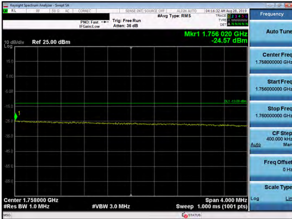
Plot 7-155. Upper Extended Band Edge Plot (Band 4 - 20.0MHz QPSK - Full RB Configuration)
