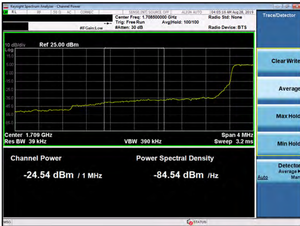
Plot 7-129. Lower Extended Band Edge Plot (Band 66/4 - 3.0MHz QPSK - Full RB Configuration)
