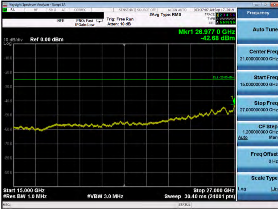
Plot 7-105. Conducted Spurious Plot (Band 7 - 20.0MHz QPSK - RB Size 1, RB Offset 0 - High Channel)
