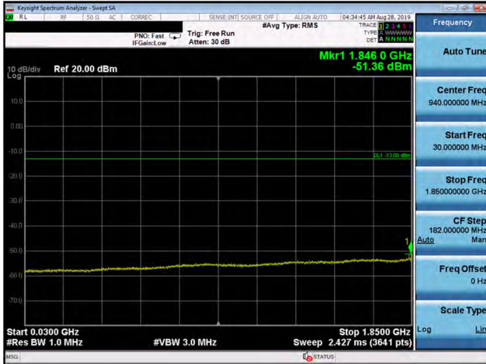
Plot 7-94. Conducted Spurious Plot (Band 2 - 20.0MHz QPSK - RB Size 1, RB Offset 0 - High Channel)
