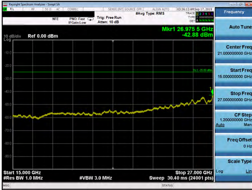
Plot 7-99. Conducted Spurious Plot (Band 7 - 20.0MHz QPSK - RB Size 1, RB Offset 0 - Low Channel)
