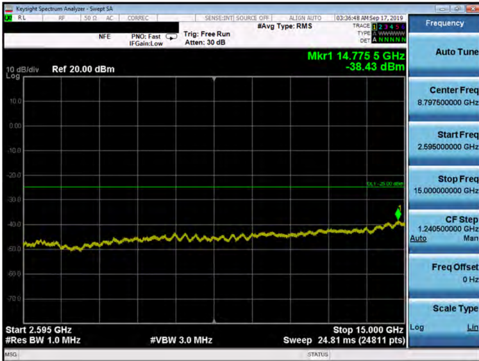
Plot 7-104. Conducted Spurious Plot (Band 7 - 20.0MHz QPSK - RB Size 1, RB Offset 0 - High Channel)
