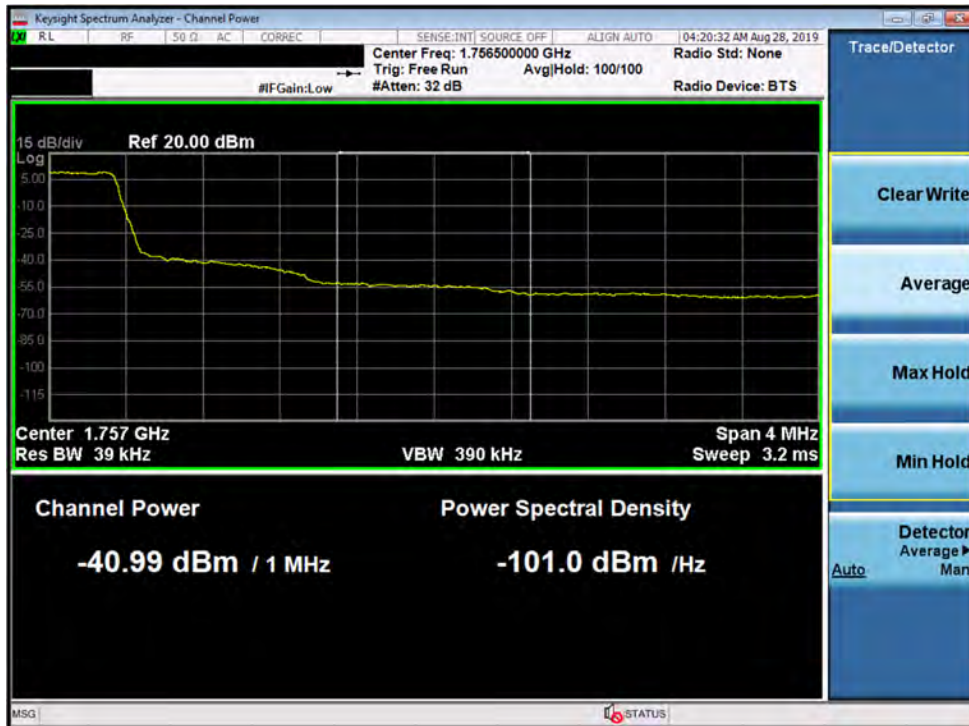
Plot 7-125. Upper Extended Band Edge Plot (Band 4 - 1.4MHz QPSK - Full RB Configuration)
