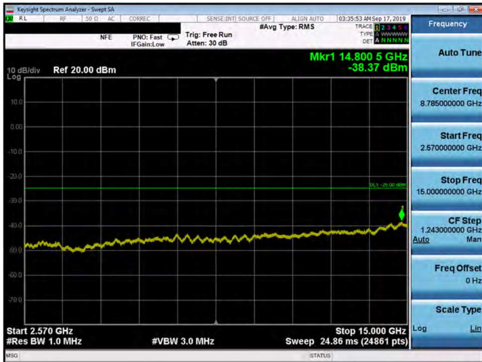
Plot 7-98. Conducted Spurious Plot (Band 7 - 20.0MHz QPSK - RB Size 1, RB Offset 0 - Low Channel)
