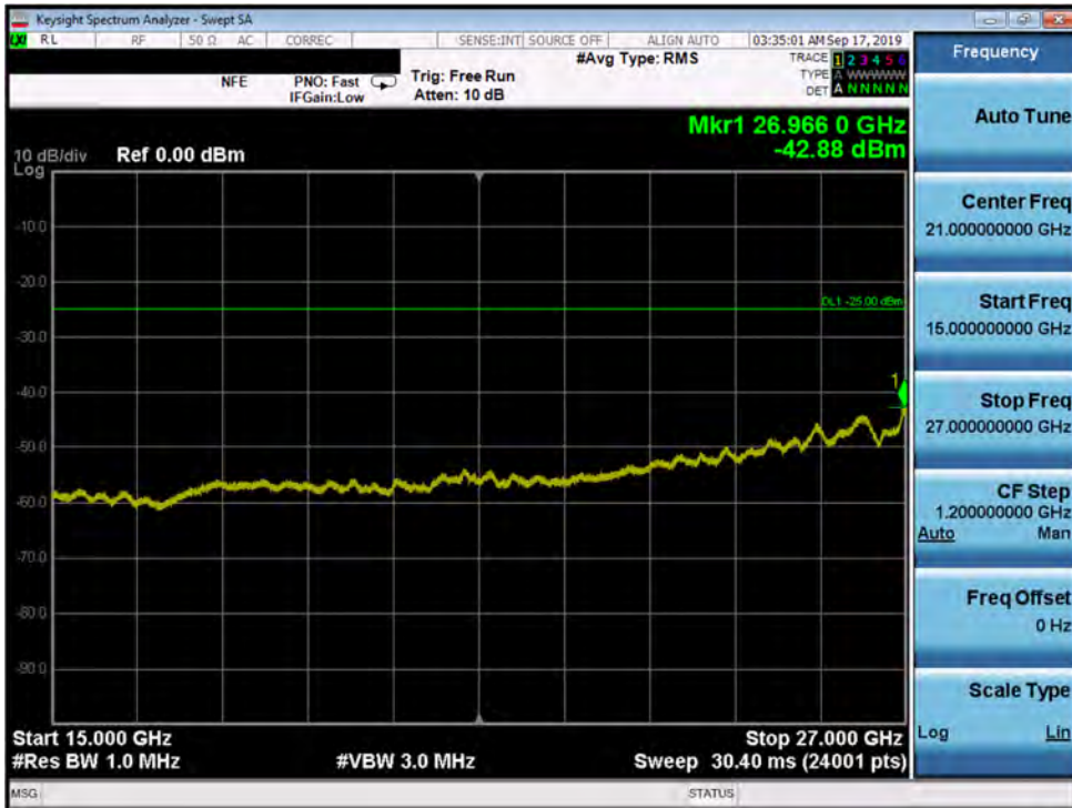
Plot 7-102. Conducted Spurious Plot (Band 7 - 20.0MHz QPSK - RB Size 1, RB Offset 0 - Mid Channel)
