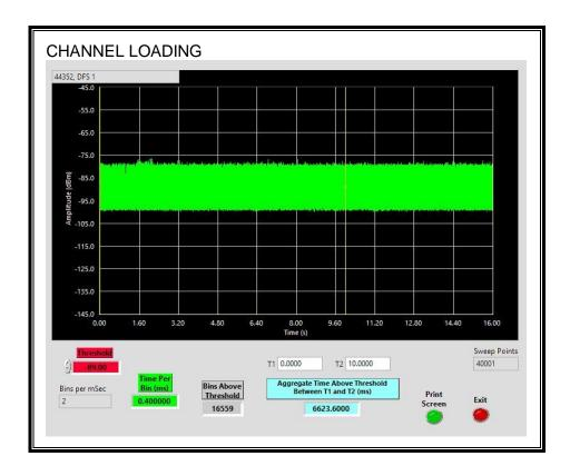
The level of traffic loading on the channel by the EUT is 66.236%.
