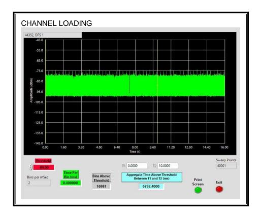
The level of traffic loading on the channel by the EUT is 67.924%.
