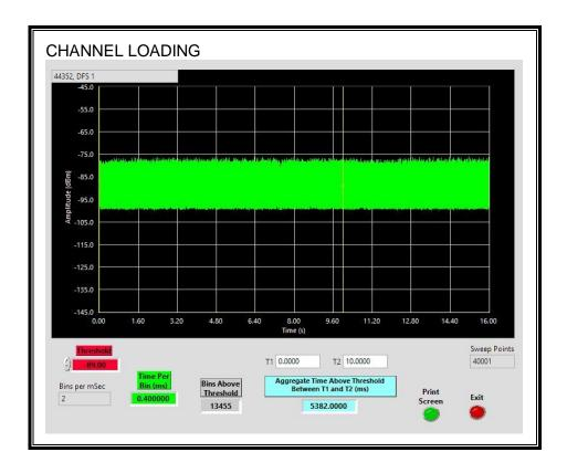
The level of traffic loading on the channel by the EUT is 53.82%.
