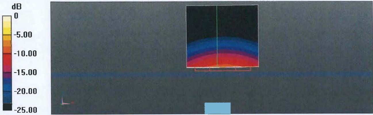
$$0 \text{ dB} = 19.3 \text{ W/kg} = 12.86 \text{ dBW/kg}$$
