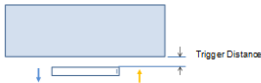
Proximity Sensor Trigger Distance Assessment KDB 616217 §6.2, Front
