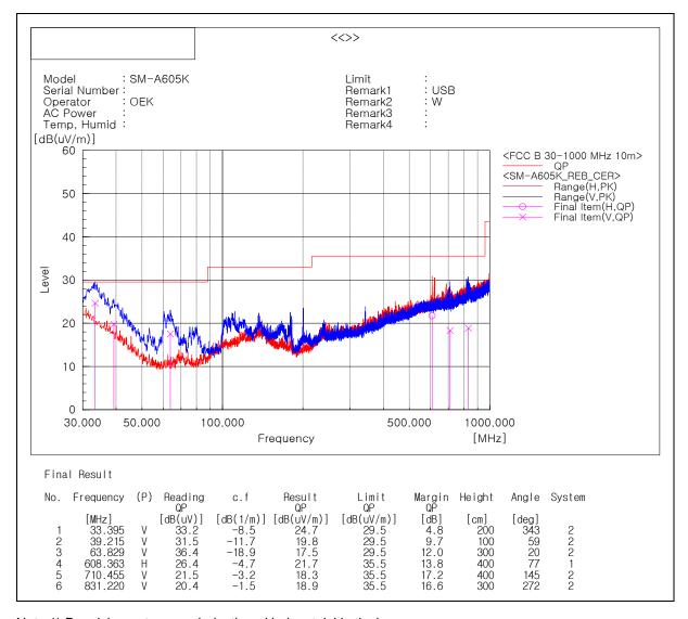
Note 1) Receiving antenna polarization : Horizontal, Vertical
