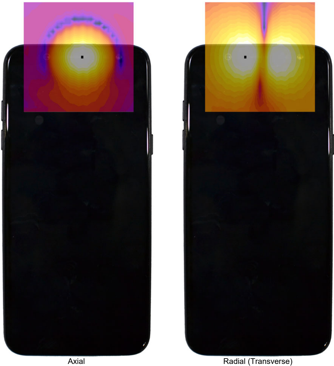
Figure 16-3 T-Coil Scan Overlay Magnetic Field Distributions
