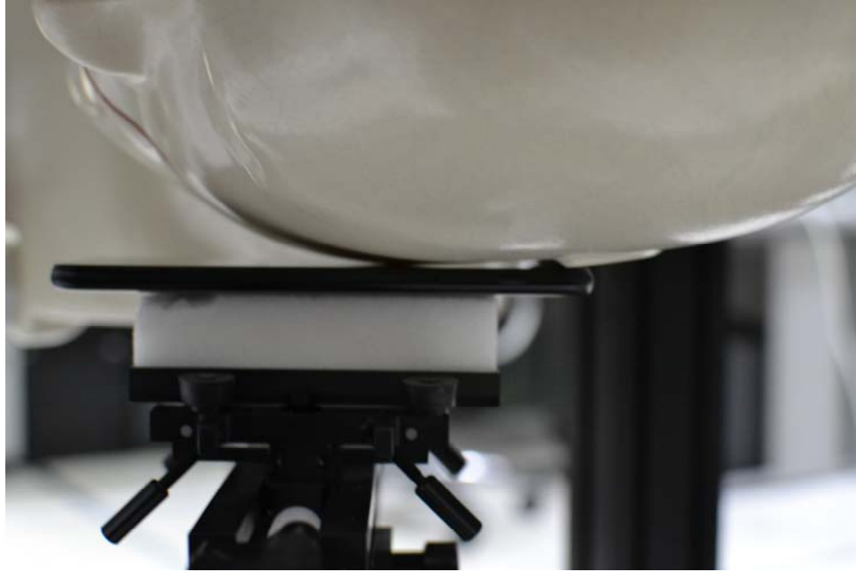
SAR Test Setup Photo 3 – Left Cheek
