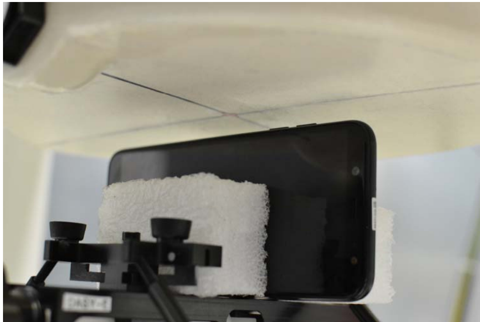
SAR Test Setup Photo 12 - Left Side at 10 mm
