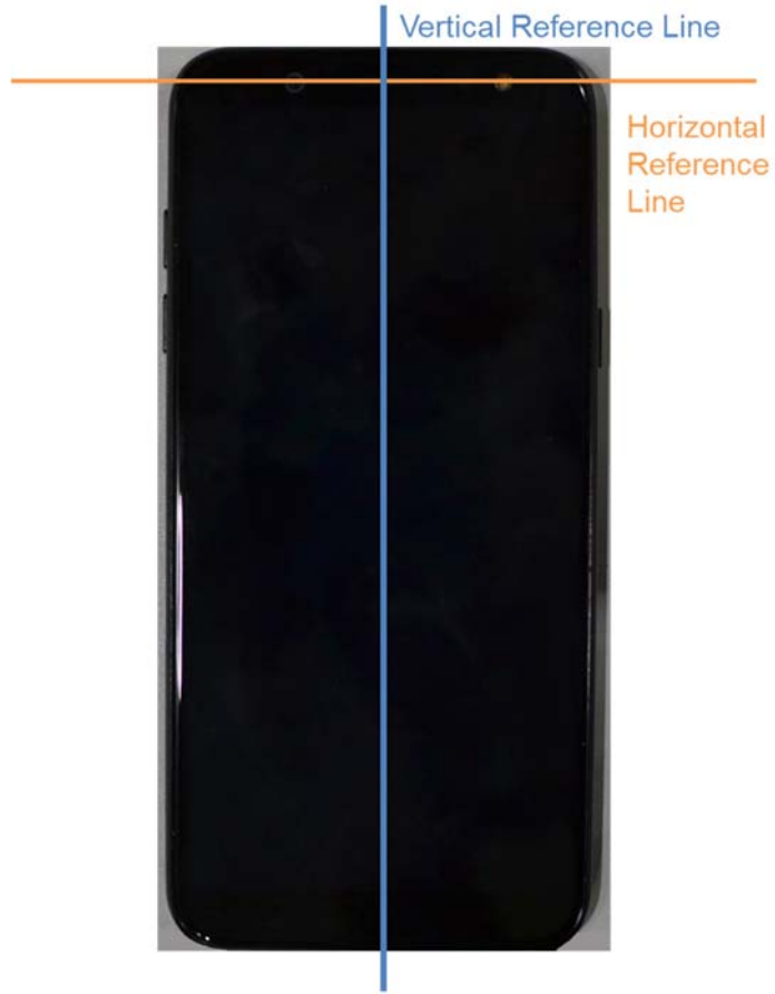
SAR Test Setup Photo 13 – Horizontal and Vertical Reference Lines
