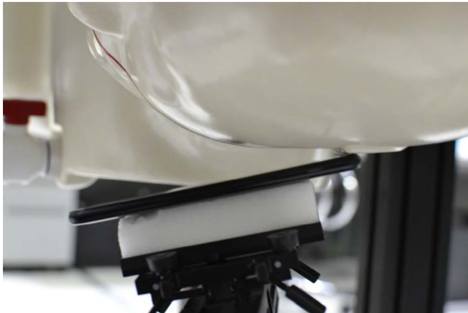
SAR Test Setup Photo 4 – Left Tilt
