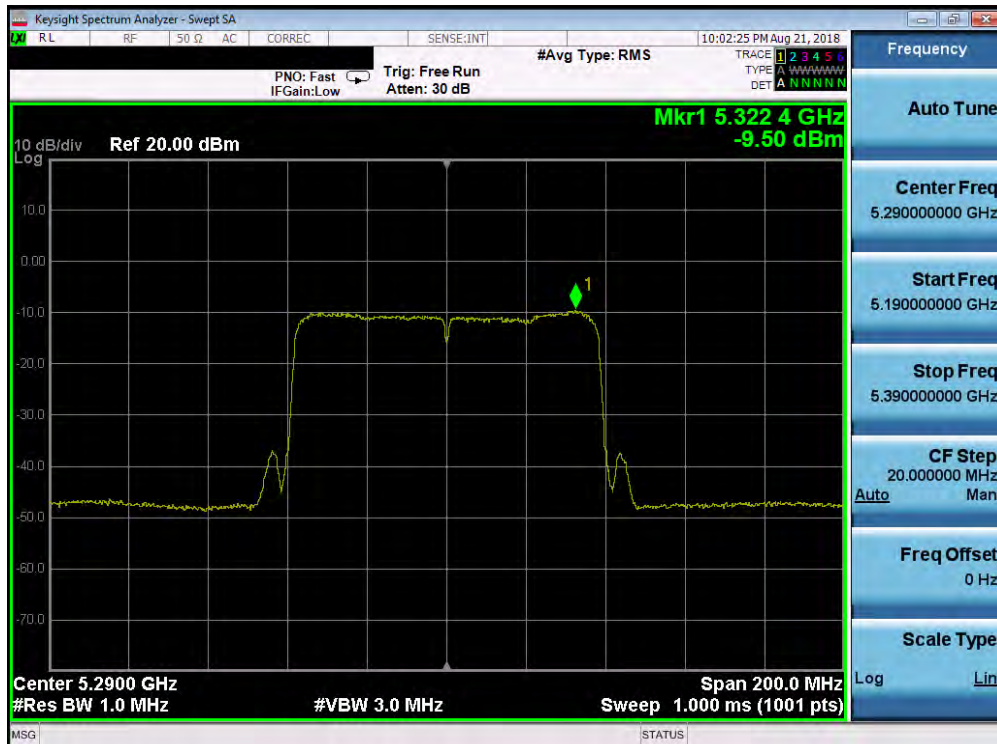
Plot 7-57. Power Spectral Density Plot (80MHz BW 802.11ac (UNII Band 2A) – Ch. 58)
