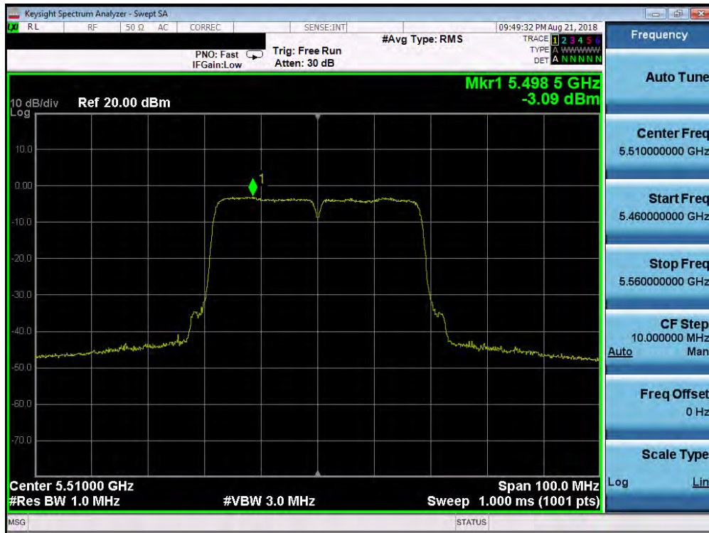
Plot 7-64. Power Spectral Density Plot (40MHz BW 802.11n (UNII Band 2C) – Ch. 102)
