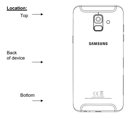
FCC ID is engraved on rear bottom of the device.
