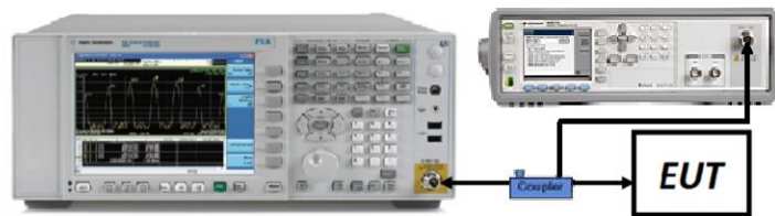
Figure 7-6. Test Instrument & Measurement Setup
