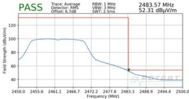
Plot 7-41. Radiated Restricted Upper Band Edge Measurement (Average)
