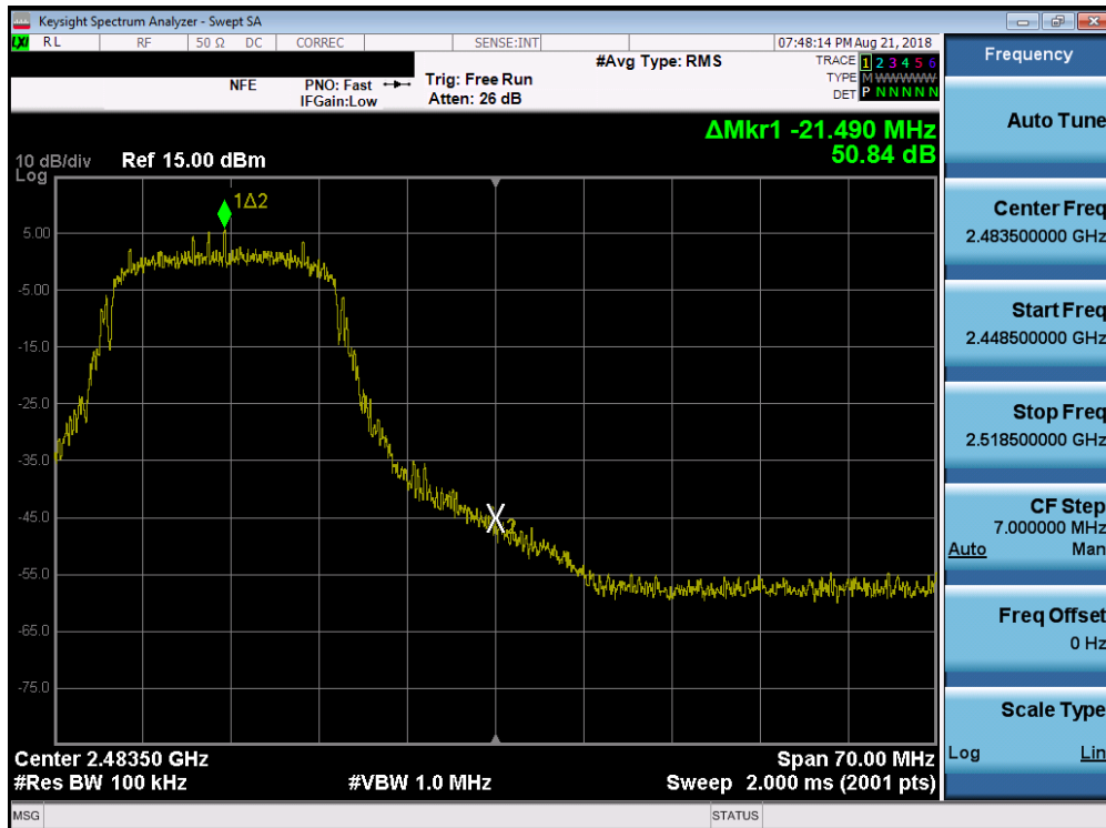
Plot 7-24. Band Edge Plot (802.11n (2.4GHz) – Ch. 11)
