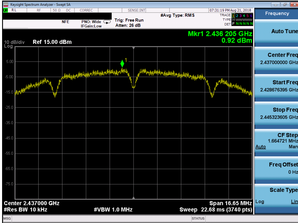
Plot 7-11. Power Spectral Density Plot (802.11b – Ch. 6)
