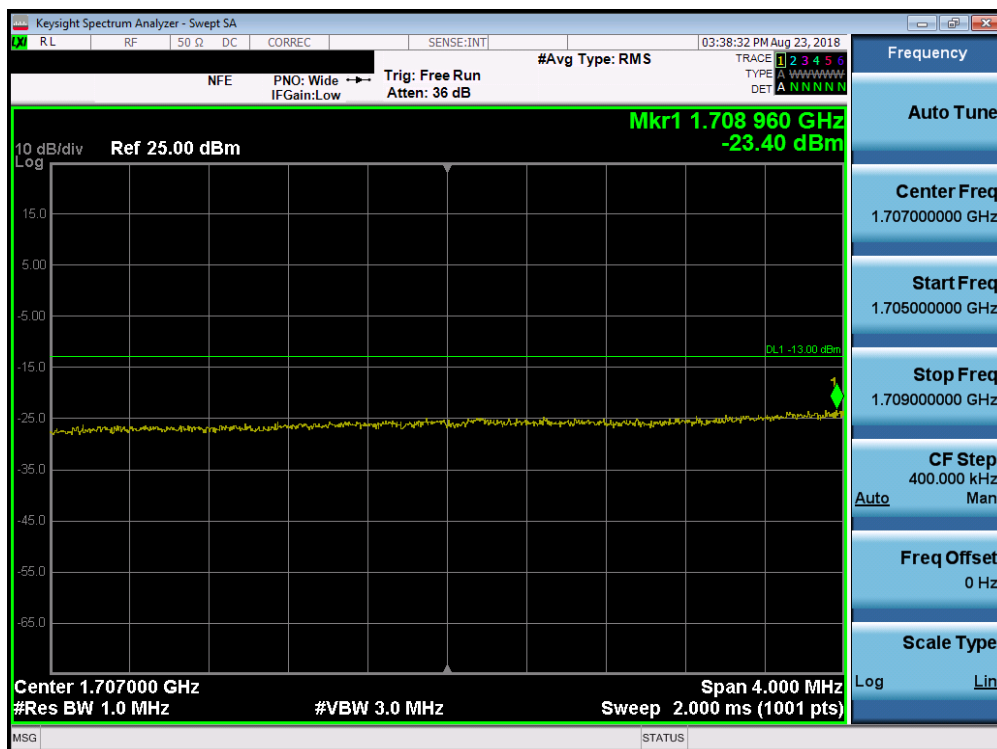
Plot 7-157. Lower Extended Band Edge Plot (Band 66/4 - 15.0MHz QPSK - Full RB Configuration)
