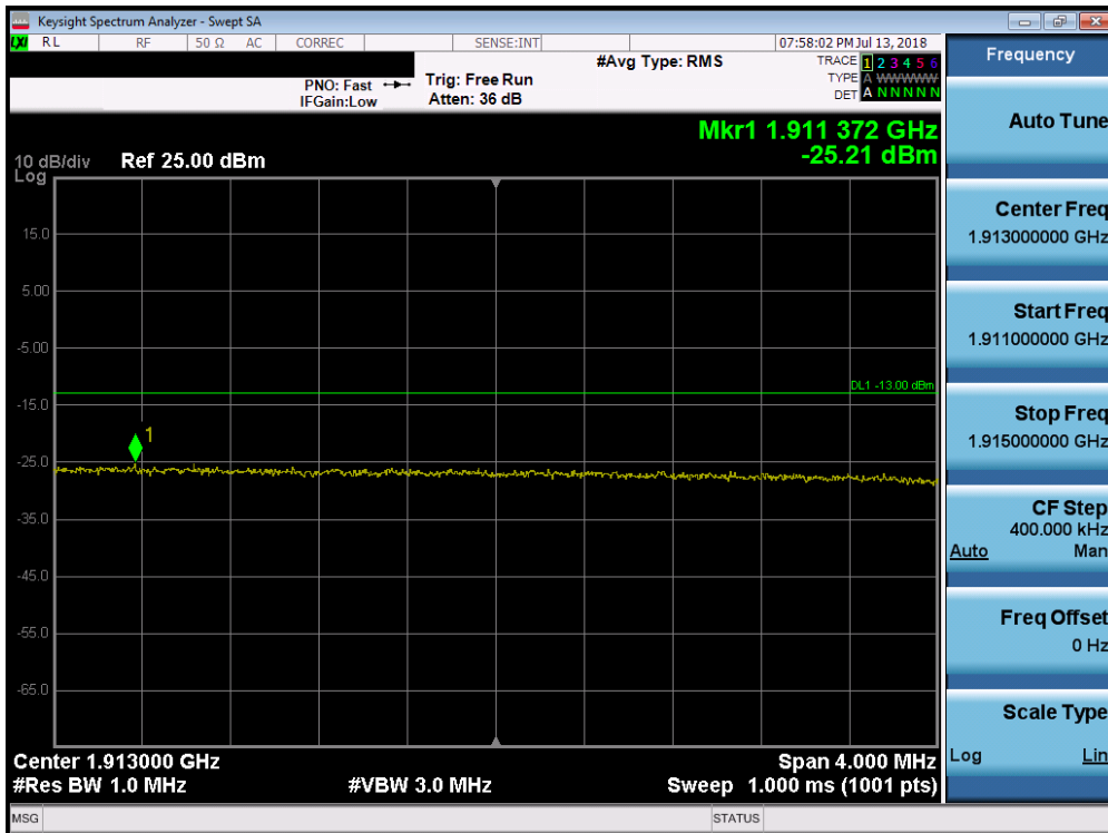
Plot 7-191. Upper Extended Band Edge Plot (Band 2 - 20.0MHz QPSK - Full RB Configuration)
