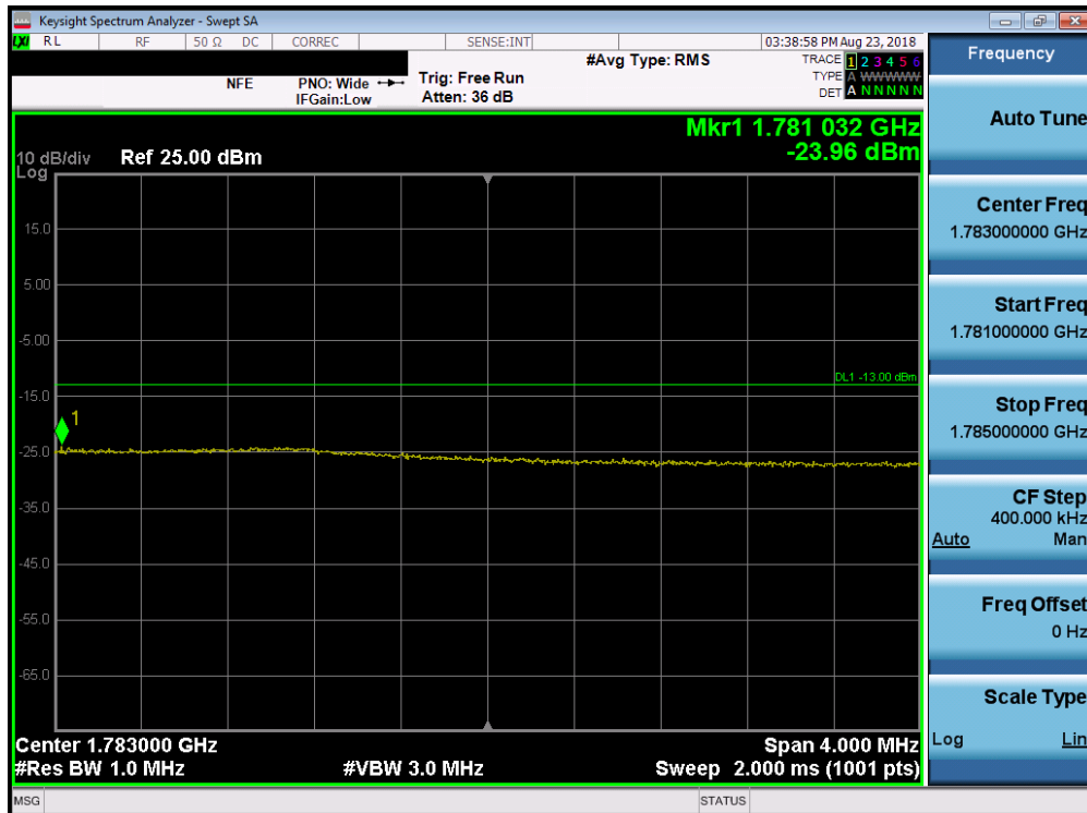
Plot 7-159. Upper Extended Band Edge Plot (Band 66 - 15.0MHz QPSK - Full RB Configuration)
