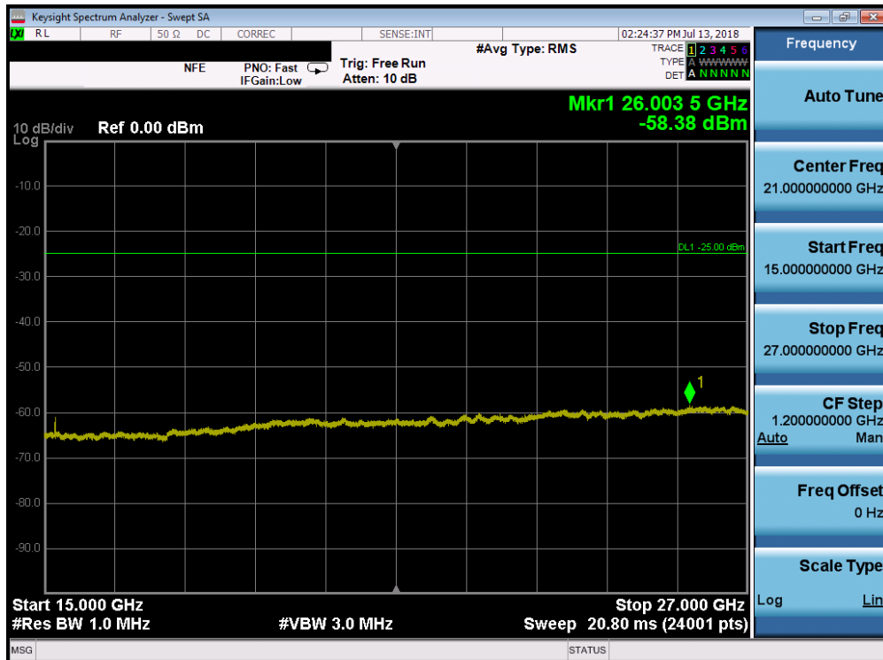
Plot 7-104. Conducted Spurious Plot (Band 7 - 10.0MHz QPSK - RB Size 1, RB Offset 0 - Mid Channel)
