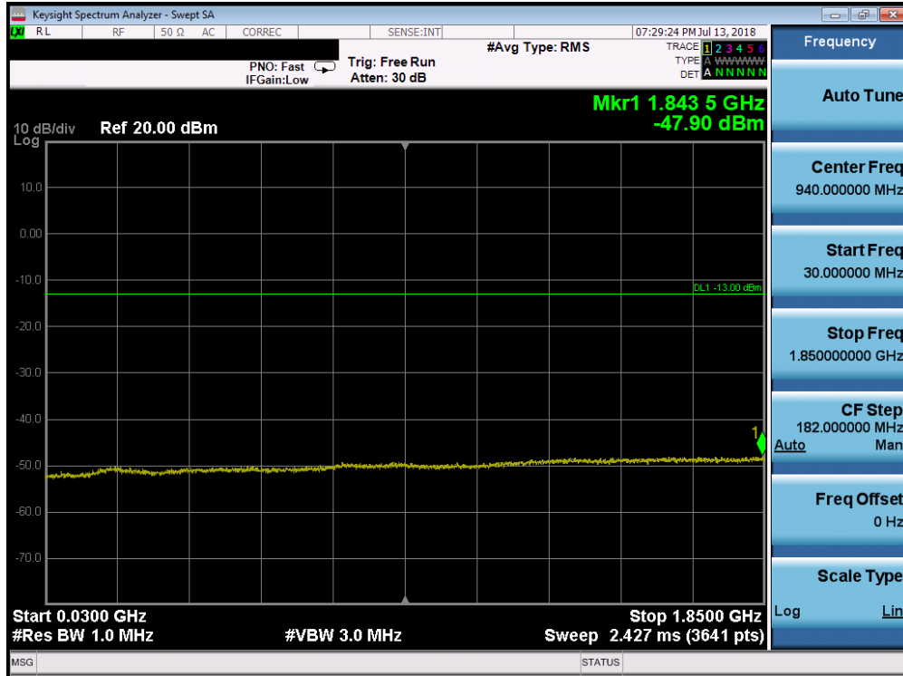
Plot 7-96. Conducted Spurious Plot (Band 2 - 10.0MHz QPSK - RB Size 1, RB Offset 0 - High Channel)
