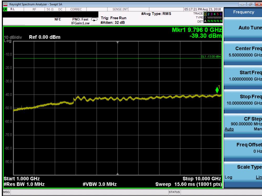
Plot 7-65. Conducted Spurious Plot (Band 71 - 20.0MHz QPSK - RB Size 1, RB Offset 0 - High Channel)
