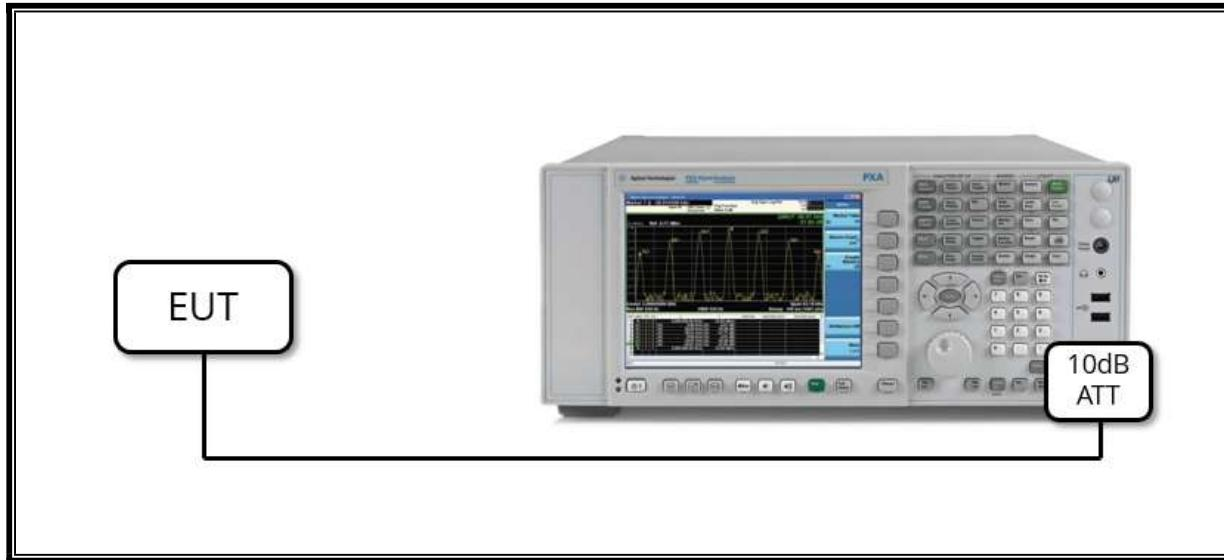
**SETUP DIAGRAM FOR TESTS (RADIATED TEST SETUP)**
