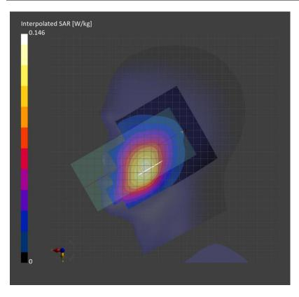
Measurement Report for SM-A556E\_DS, Rear, Band 5, LTE-FDD (SC-FDMA, 1 RB, 10 MHz, QPSK) RBPosition:Mid AntennaCfg:SISO, Channel 20525 (836.5 MHz)
