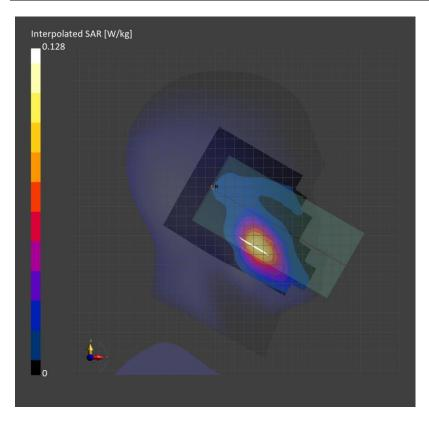
Measurement Report for SM-A556E\_DS, BOTTOM, Band n66, 5G NR (DFT-s-OFDM, 50% RB, 40 MHz, QPSK, 15 kHz) RBPosition:Mid AntennaCfg:SISO, Channel 349000 (1745.0 MHz)
