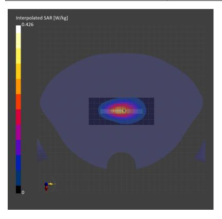
Measurement Report for SM-A556E\_DS, Right Touch, Band n5, 5G NR (DFT-s-OFDM, 50% RB, 20 MHz, QPSK, 15 kHz) RBPosition:Mid AntennaCfg:SISO, Channel 167300 (836.5 MHz)
