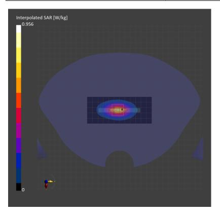
Measurement Report for SM-A556E\_DS, RIGHT TILT, Band n66, 5G NR (DFT-s-OFDM, 50% RB, 40 MHz, QPSK, 15 kHz) RBPosition:Mid AntennaCfg:SISO, Channel 349000 (1745.0 MHz)
