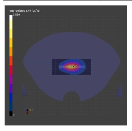
Measurement Report for SM-A556E\_DS, RIGHT TILT, Band n77, 5G NR (DFT-s-OFDM, 1 RB, 100 MHz, QPSK, 30 kHz) RBPosition:High AntennaCfg:SISO, Channel 662000 (3930.0 MHz)
