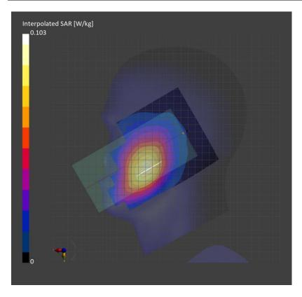
Measurement Report for SM-A556E\_DS, Rear, Band 12, LTE-FDD (SC-FDMA, 1 RB, 10 MHz, QPSK) RBPosition:Mid AntennaCfg:SISO, Channel 23095 (707.5 MHz)
