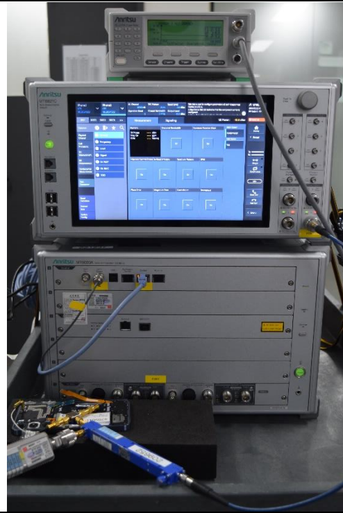
A.4 F_TC 02/04/13 Conducted test in MT8000A callbox
