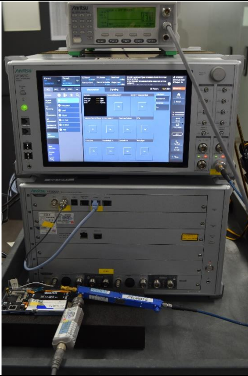
A.3 F_TC 15 Conducted test in MT8821C callbox
