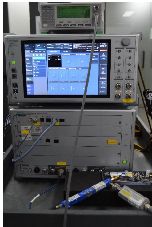
A.4 F_TC 02/04/13 Conducted test in MT8000A callbox
