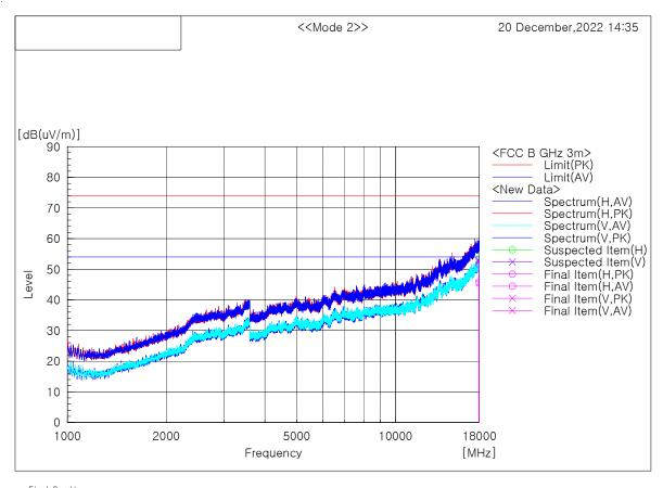
Final Result Margin PK [dB] 22.4 21.6 Margin Height AV [dB] [cm] 8.3 99.7 8.5 99.7 No. Frequency (P) Reading [MHz] 17986.500
