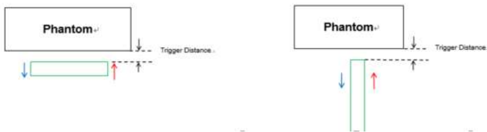
Proximity Sensor Trigger Distance Assessment KDB 616217 D04§6.2 (Rear / Front / Bottom side)
