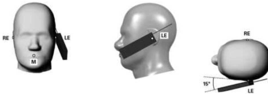
Figure 8.5. Tilt 15° position of the wireless device
