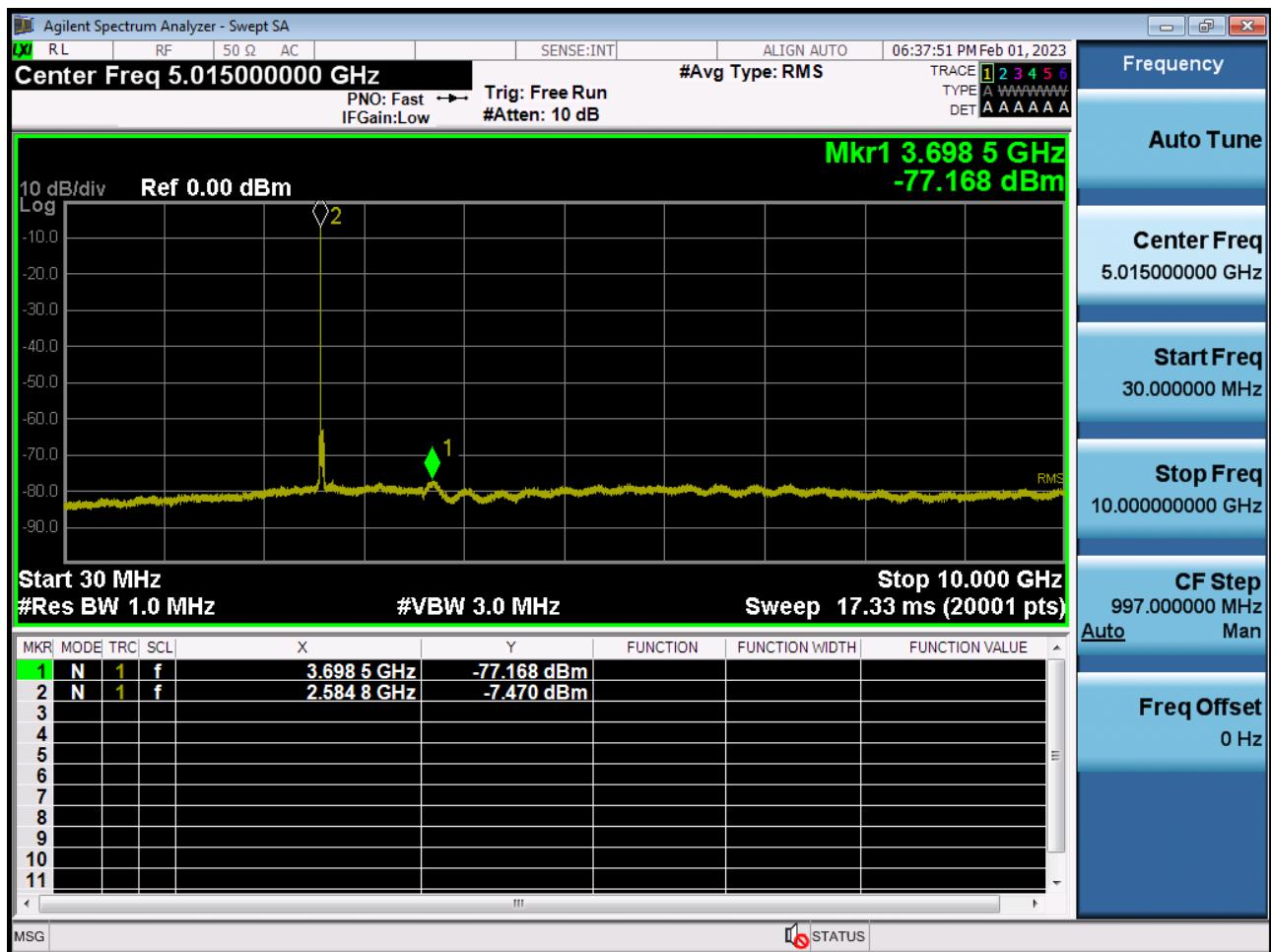
Conducted Spurious Plot 2 (20 MHz Ch. 40620 QPSK RB 1, Offset 0)
