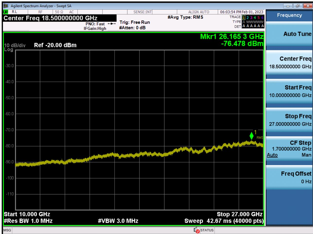
Conducted Spurious Plot 1 (5 MHz Ch.40620 QPSK RB 1, Offset 0)
