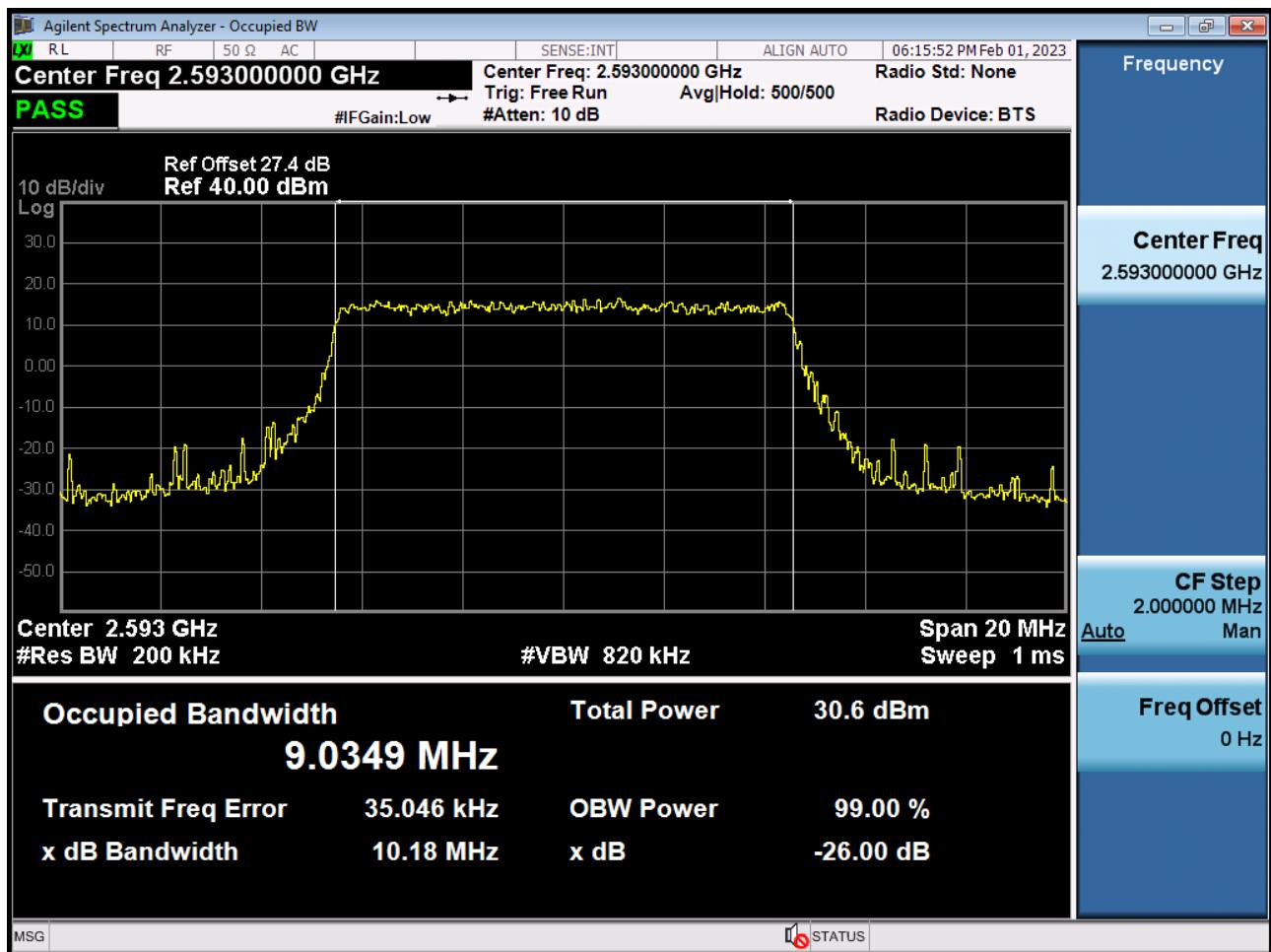
Occupied Bandwidth Plot (10 MHz Ch.40620 16-QAM RB 50)
