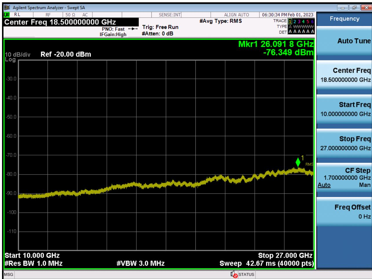
Conducted Spurious Plot 1 (20 MHz Ch.39750 QPSK RB 1, Offset 0)
