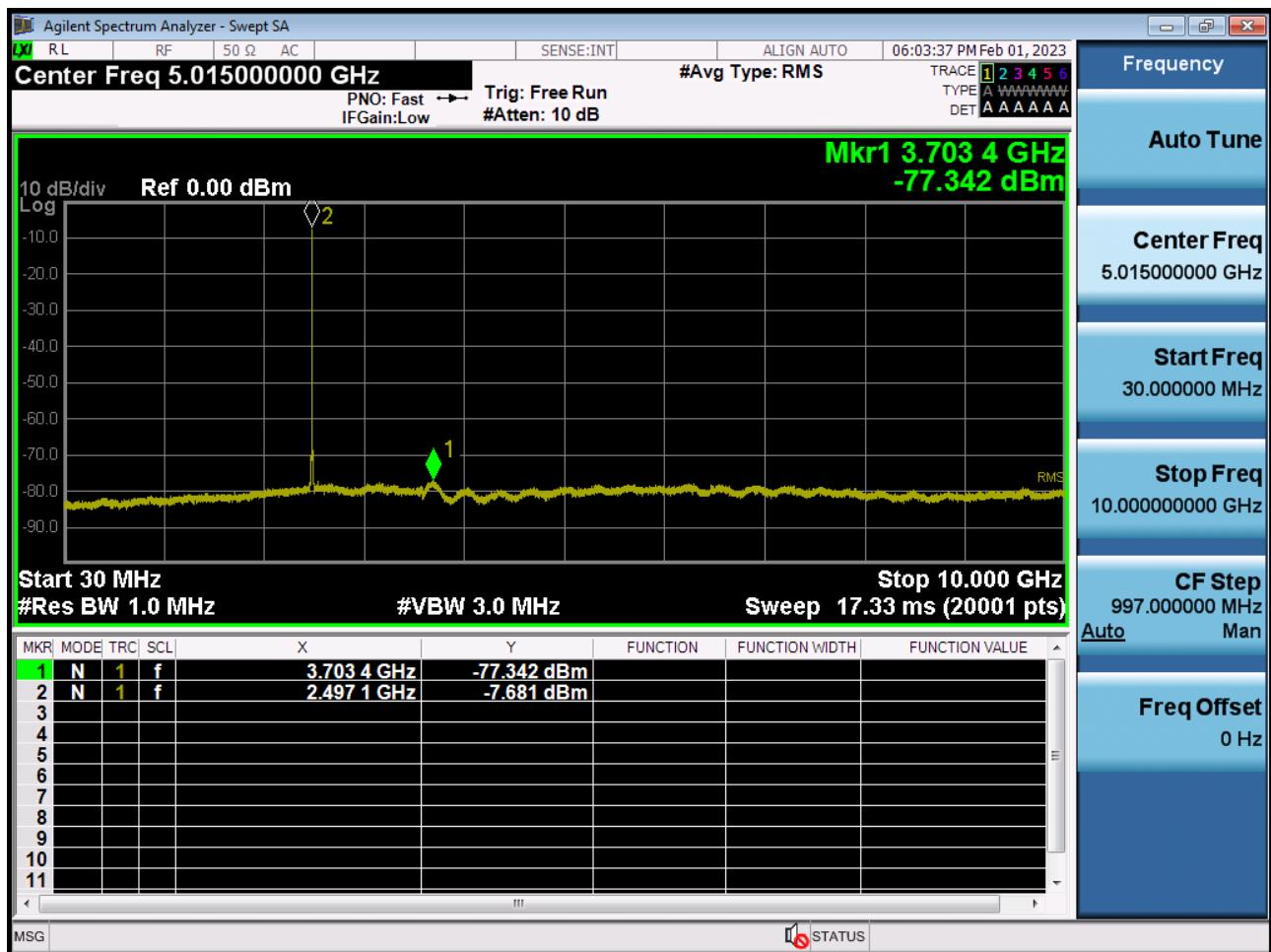
Conducted Spurious Plot 2 (5 MHz Ch. 39675 QPSK RB 1, Offset 0)
