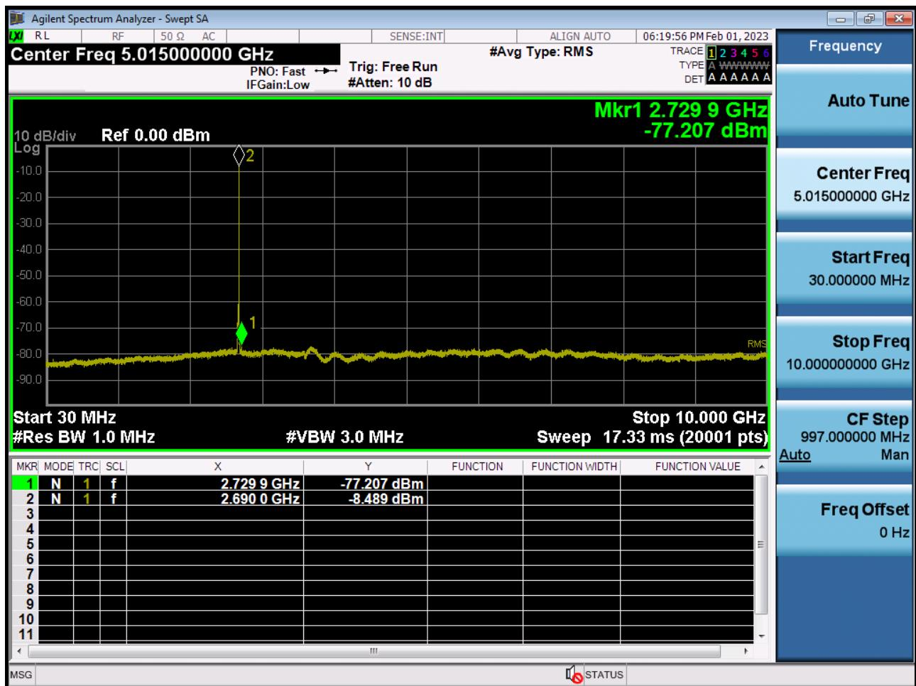
Conducted Spurious Plot 2 (10 MHz Ch. 41540 QPSK RB 1, Offset 0)
