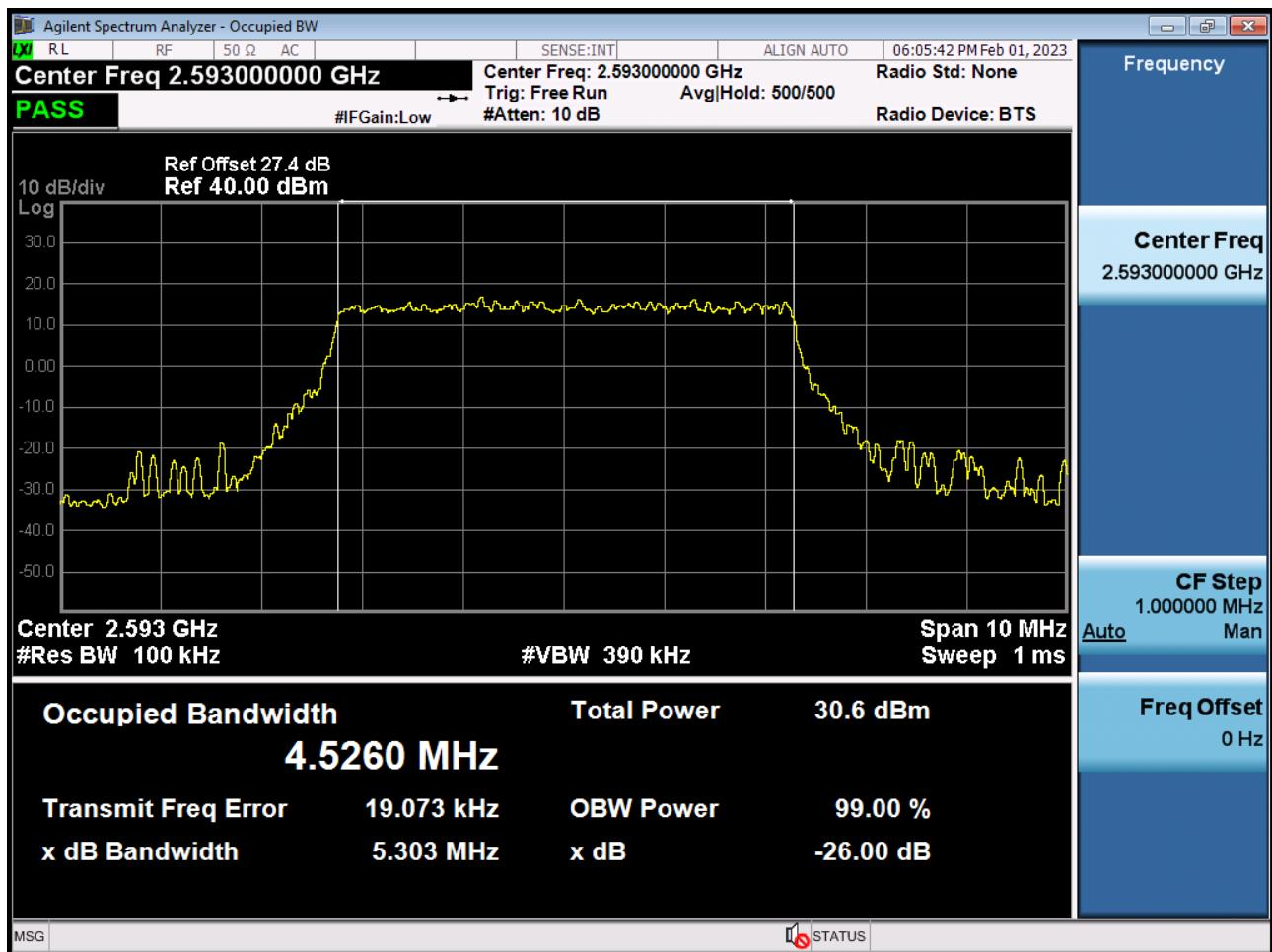
Occupied Bandwidth Plot (5 MHz Ch.40620 16-QAM RB 25)
