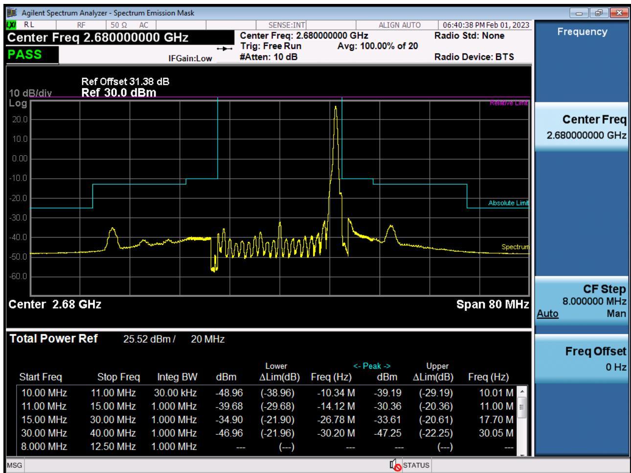
High Channel Edge Plot (20 MHz Ch.41490 QPSK\_RB100\_Offset 0)
