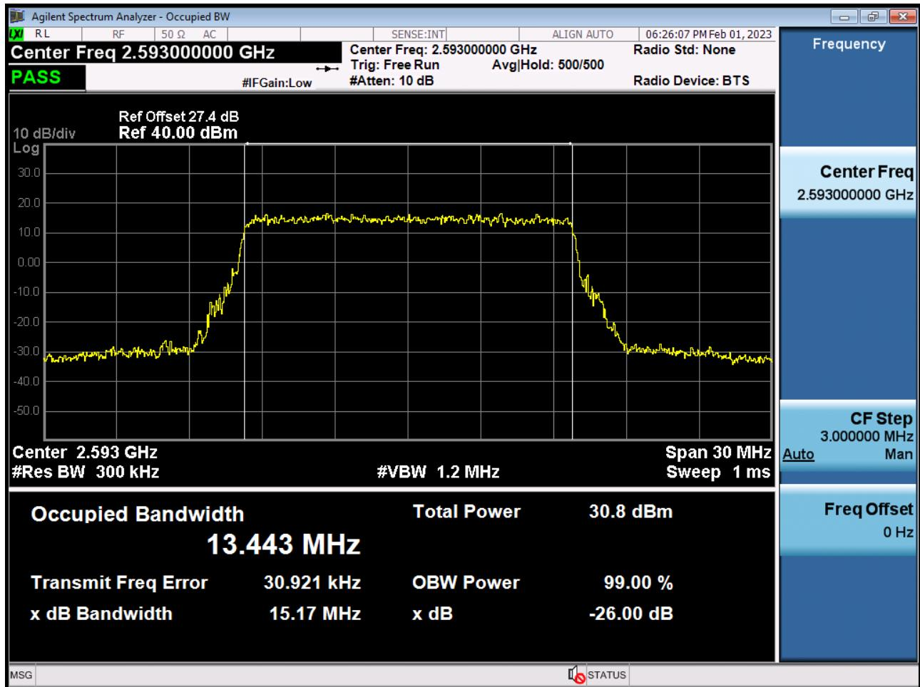
Occupied Bandwidth Plot (15 MHz Ch.40620 16-QAM RB 75)
