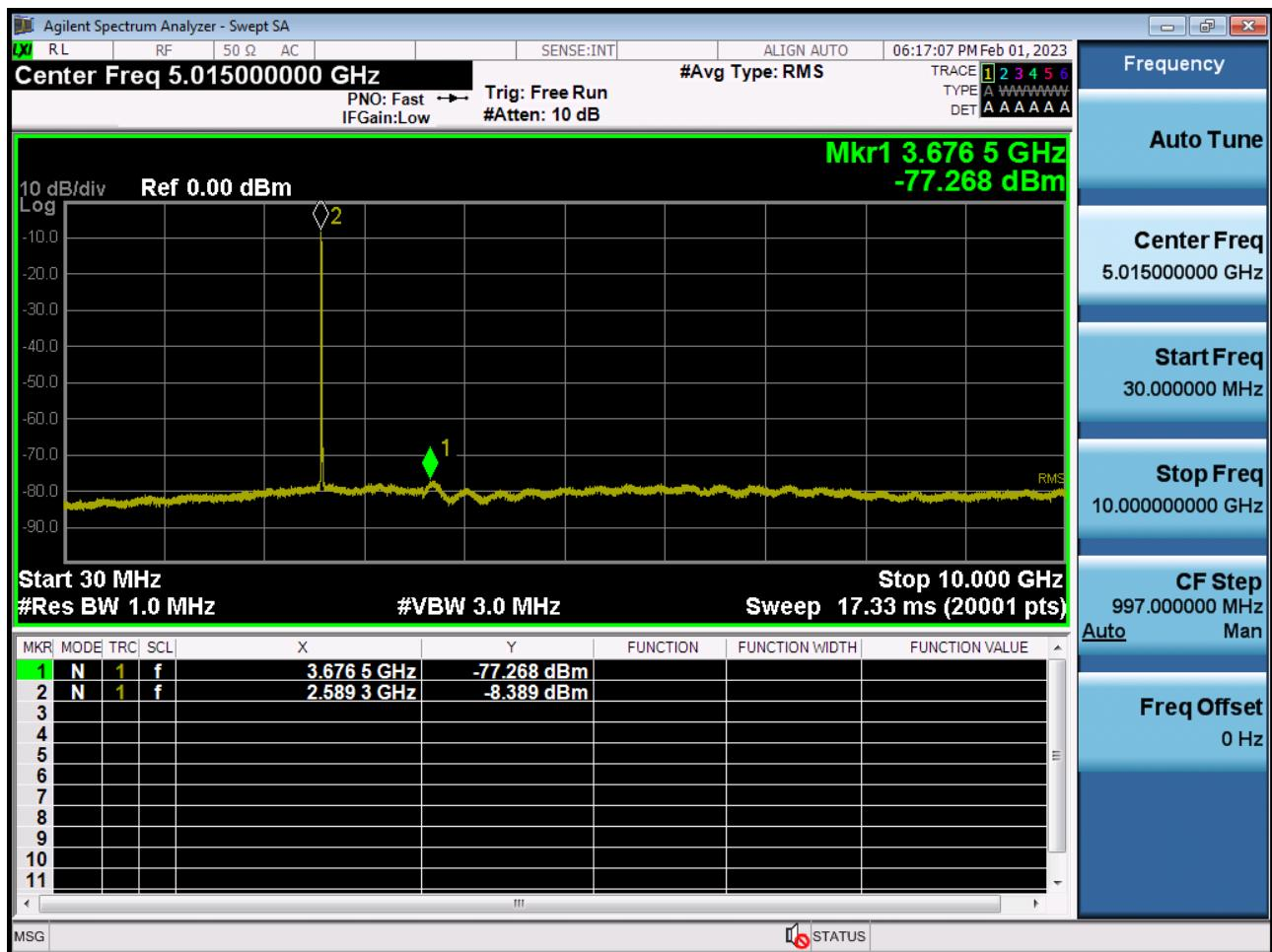
Conducted Spurious Plot 2 (10 MHz Ch. 40620 QPSK RB 1, Offset 0)
