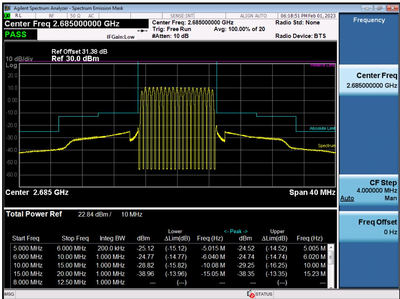
Low Channel Edge Plot (15 MHz Ch.39725 QPSK RB 1, Offset 0)-1
