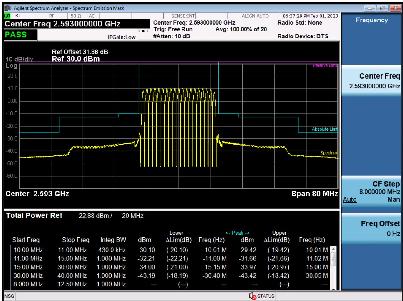
High Channel Edge Plot (20 MHz Ch.41490 QPSK RB 1, Offset 99)
