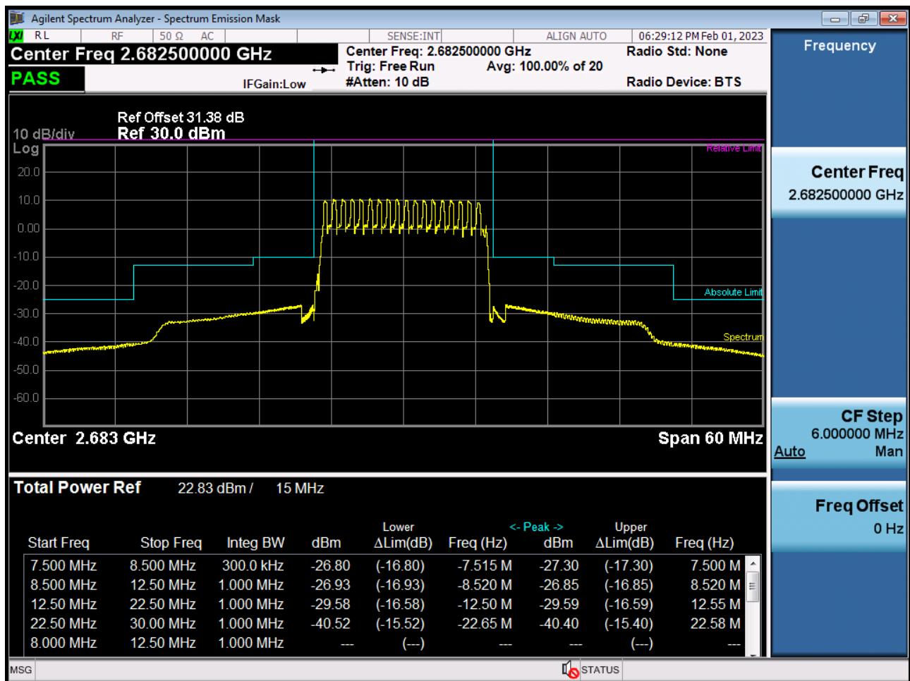
Low Channel Edge Plot (20 MHz Ch.39750 QPSK RB 1, Offset 0)-1
