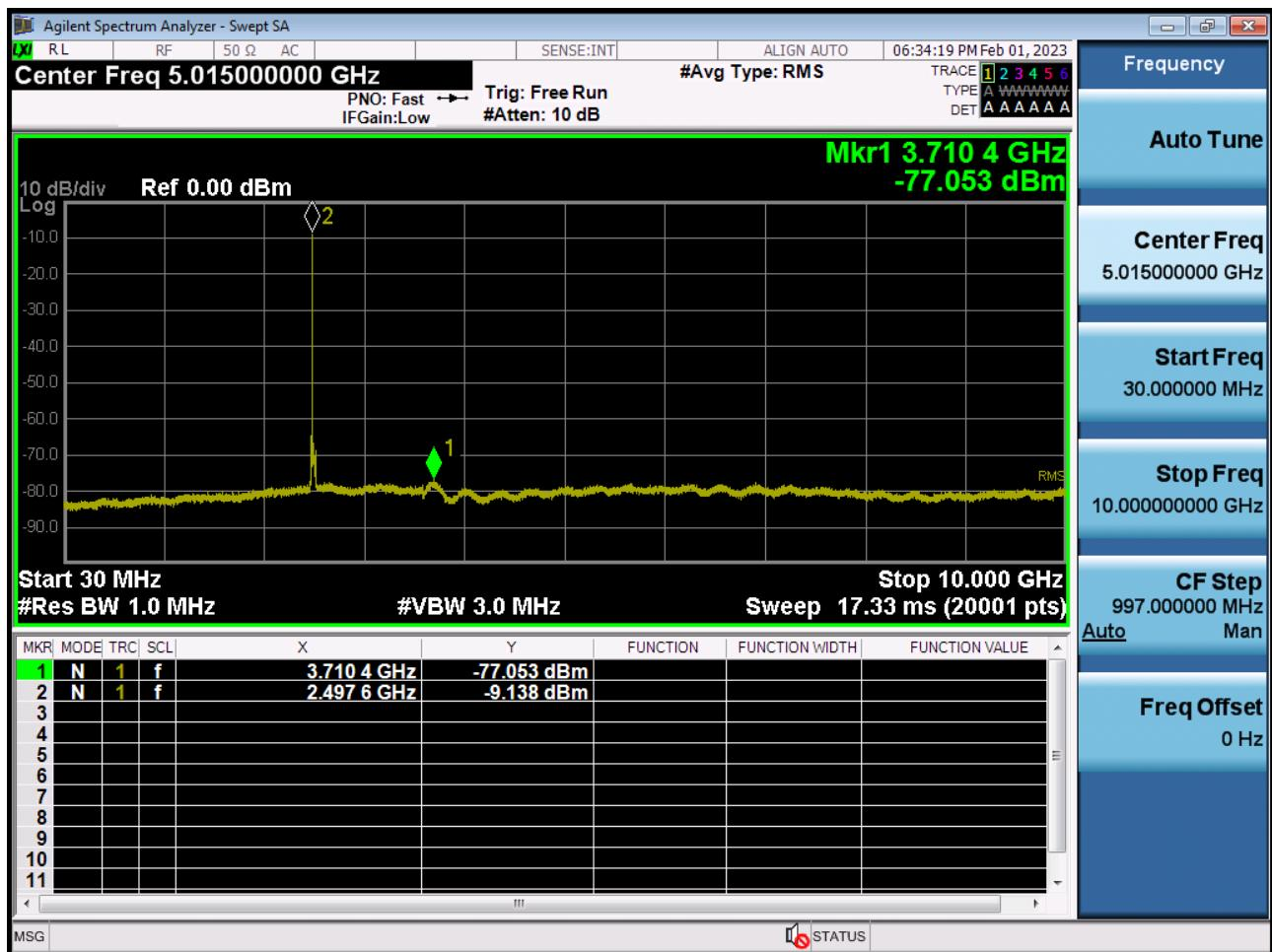
Conducted Spurious Plot 2 (20 MHz Ch. 39750 QPSK RB 1, Offset 0)
