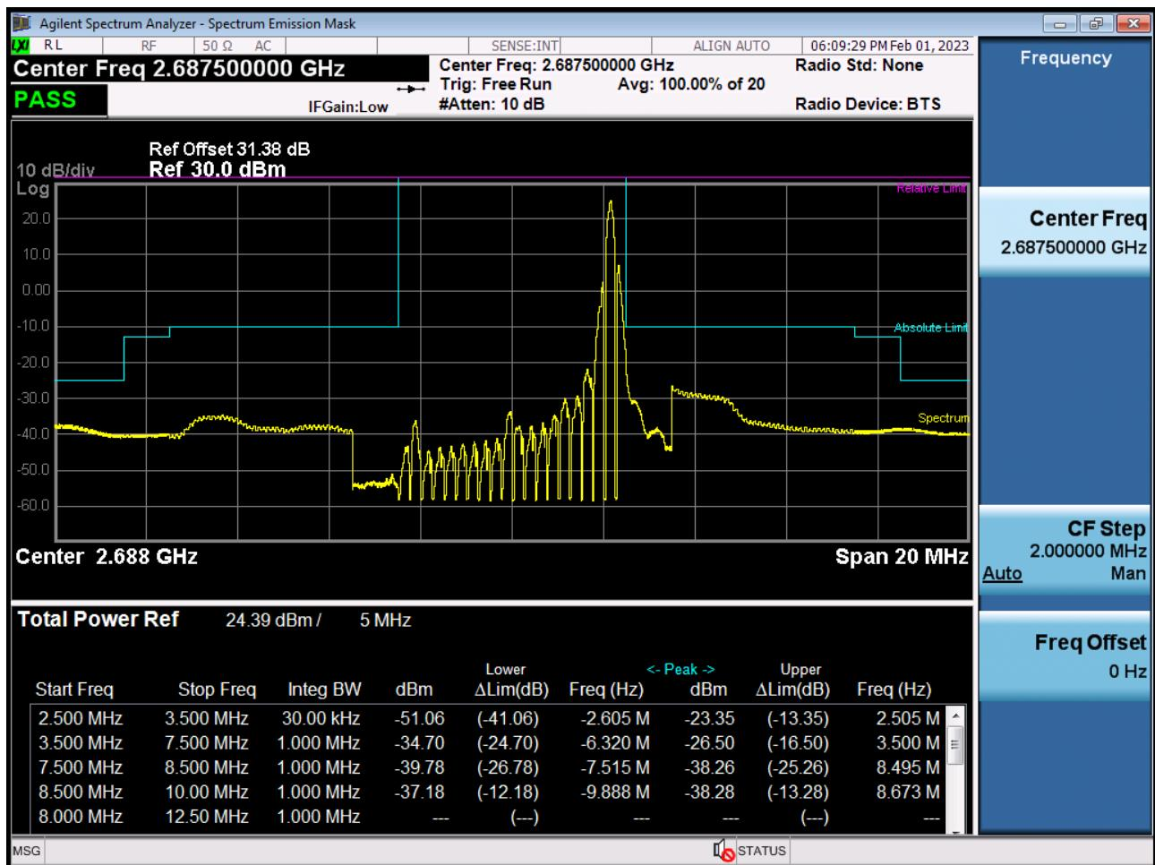
High Channel Edge Plot (5 MHz Ch.41565 QPSK\_RB25\_Offset 0)
