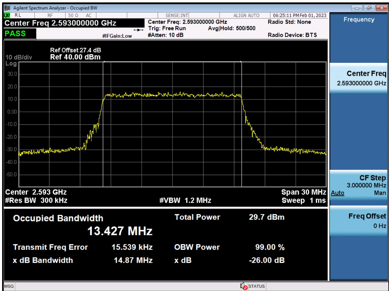
Occupied Bandwidth Plot (15 MHz Ch.40620 64-QAM RB 75)
