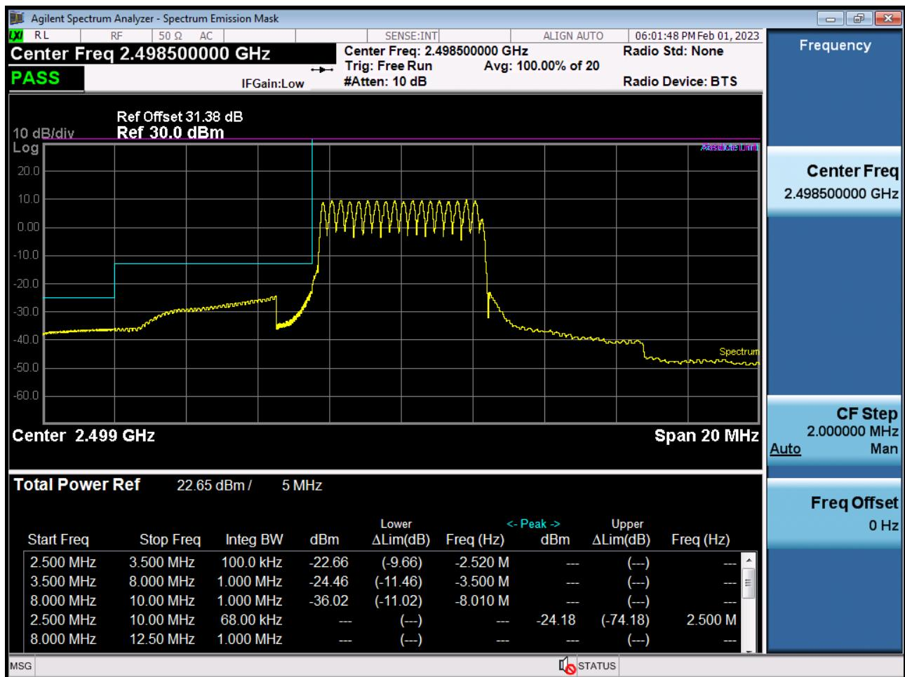
Low Channel Edge Plot (5 MHz Ch.39675 QPSK\_RB25\_Offset 0)-1
