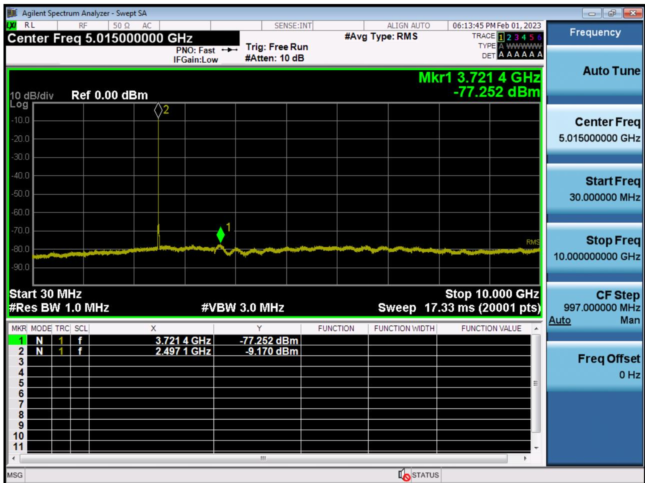
Conducted Spurious Plot 2 (10 MHz Ch. 39700 QPSK RB 1, Offset 0)
