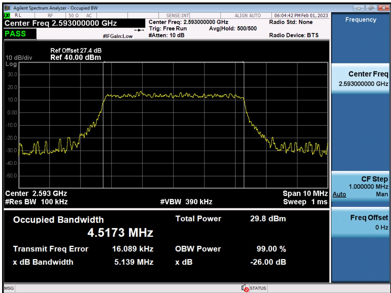
Occupied Bandwidth Plot (5 MHz Ch.40620 64-QAM RB 25)
