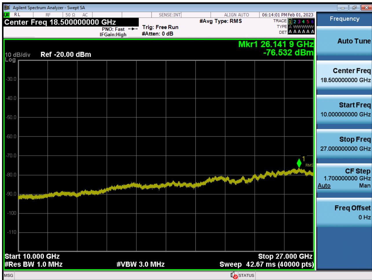
Conducted Spurious Plot 1 (10 MHz Ch.40620 QPSK RB 1, Offset 0)
