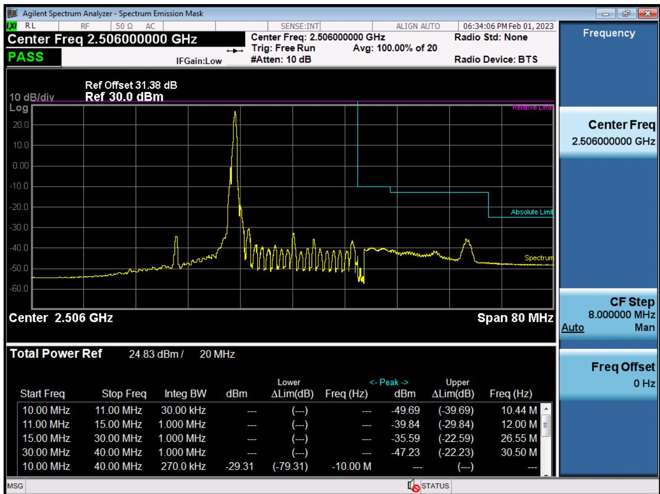
Low Channel Edge Plot (20 MHz Ch.39750 QPSK\_RB100\_Offset 0)-2
