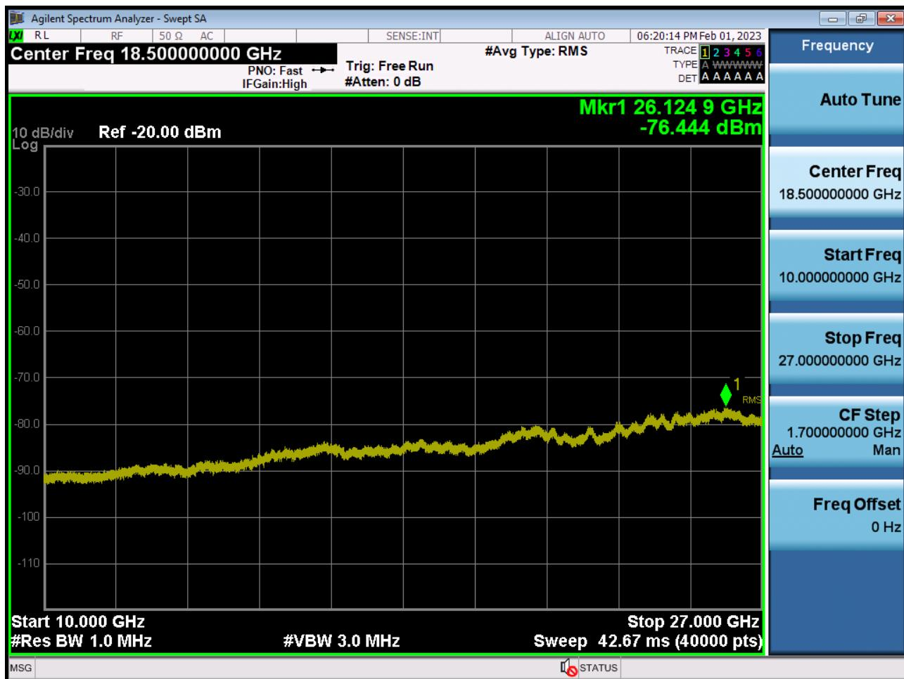
Conducted Spurious Plot 1 (15 MHz Ch.39725 QPSK RB 1, Offset 0)
