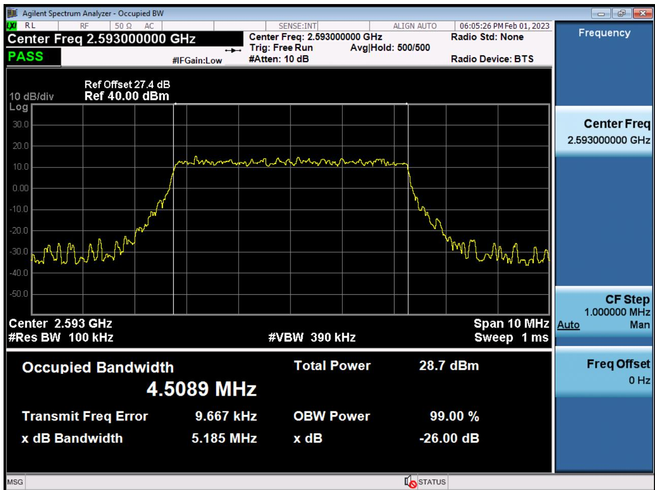
Occupied Bandwidth Plot (10 MHz Ch.40620 QPSK RB 50)
