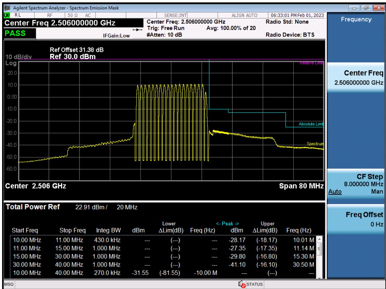
Mid Channel Edge Plot (20 MHz Ch.40620 QPSK RB 100)
