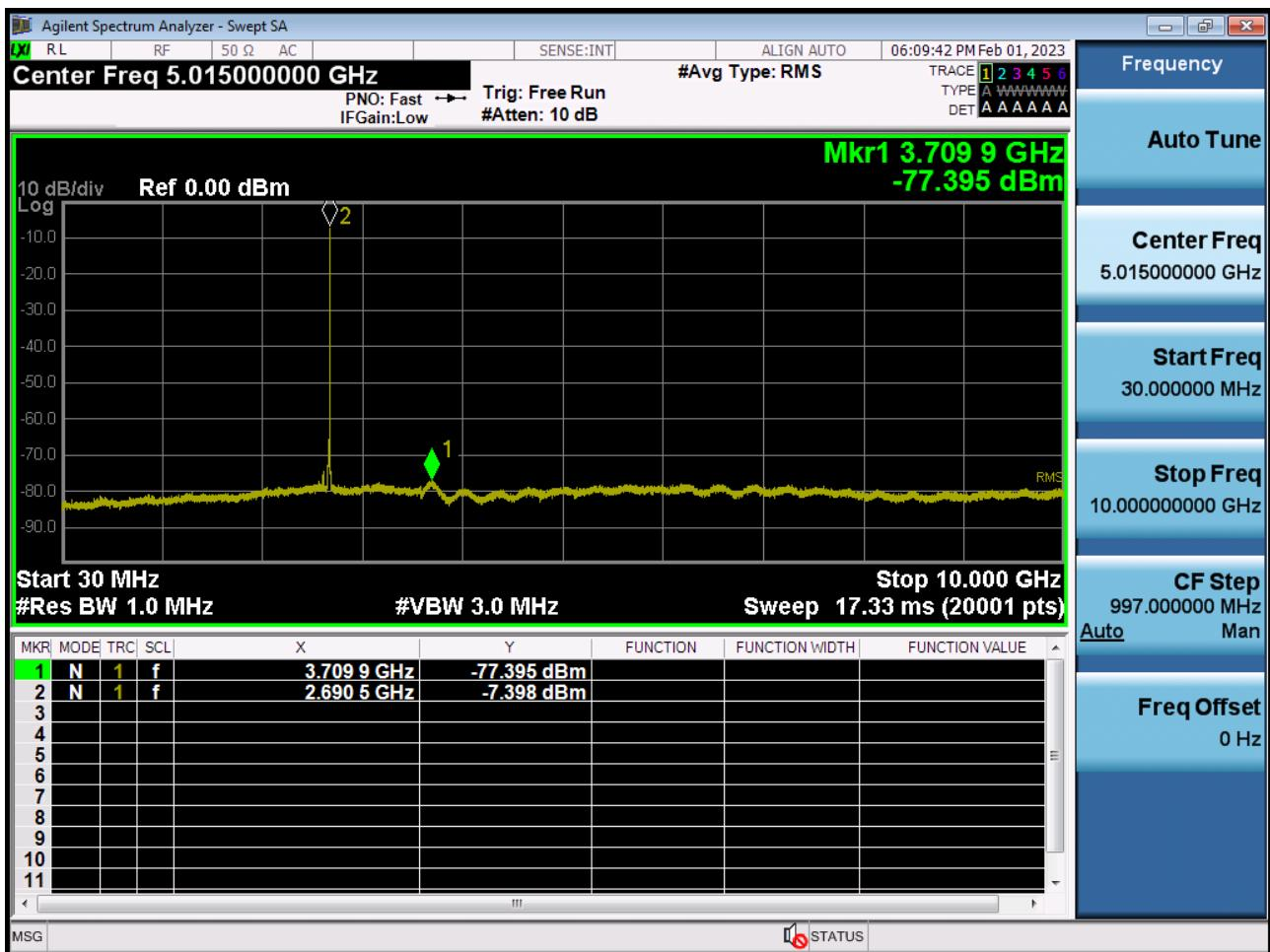
Conducted Spurious Plot 2 (5 MHz Ch. 41565 QPSK RB 1, Offset 0)
