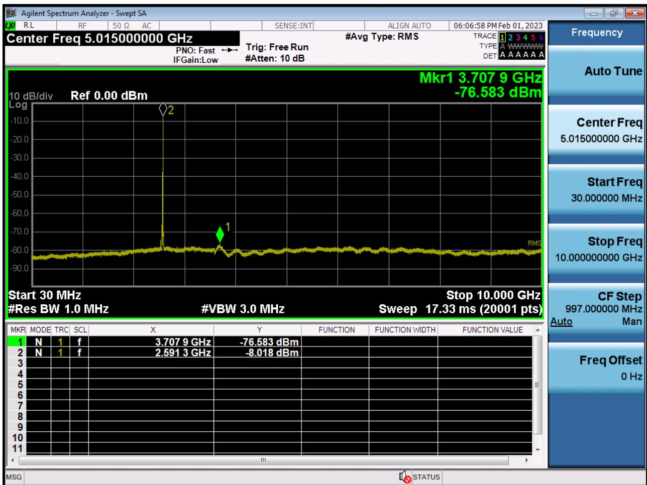
Conducted Spurious Plot 2 (5 MHz Ch. 40620 QPSK RB 1, Offset 0)
