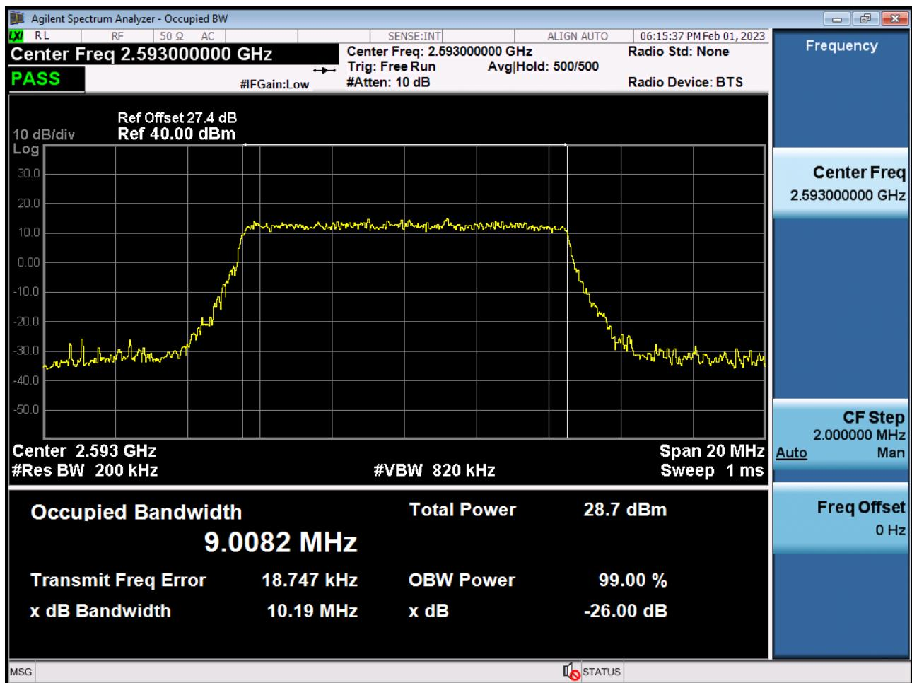
Occupied Bandwidth Plot (15 MHz Ch.40620 QPSK RB 75)
