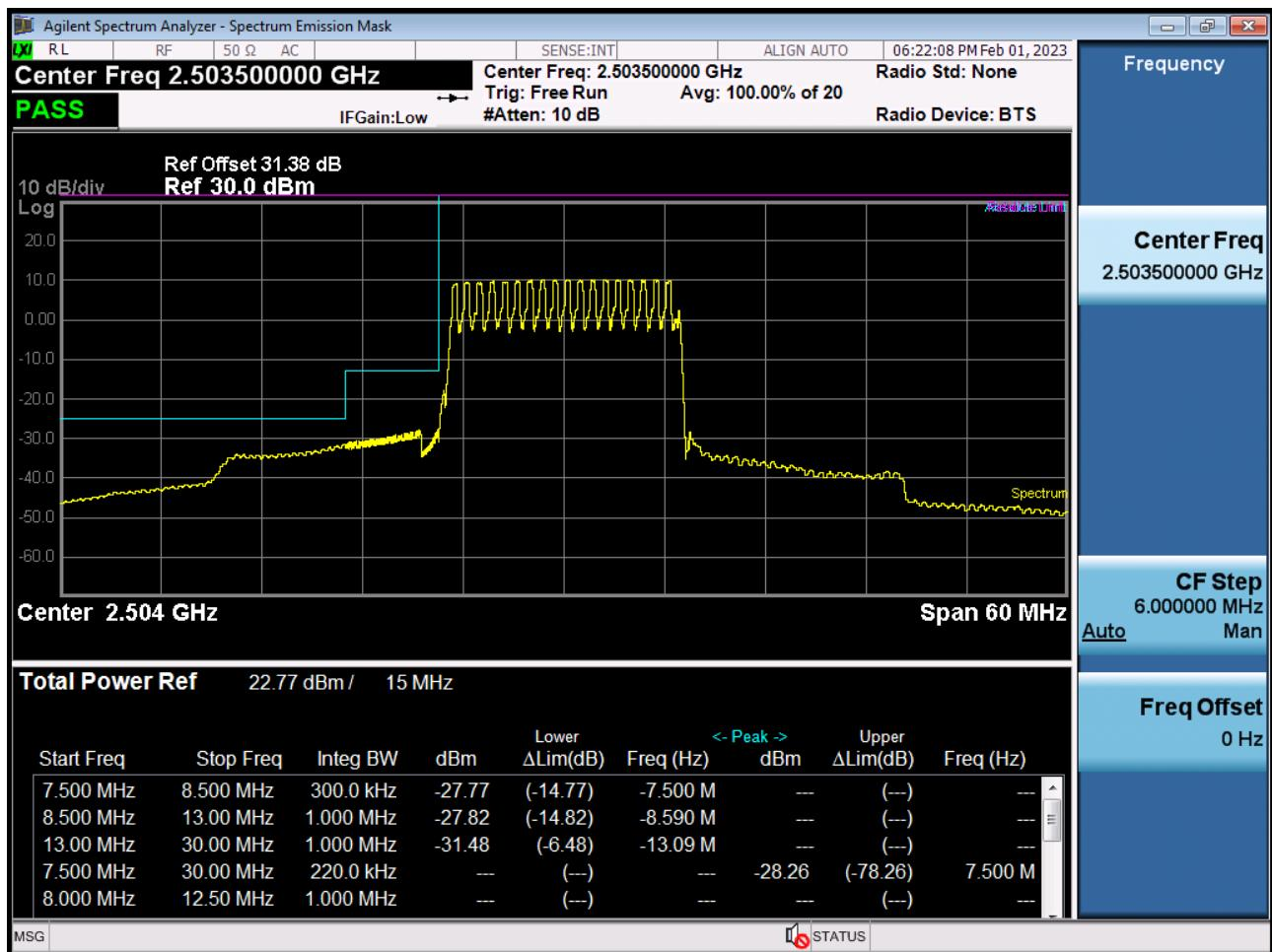
Low Channel Edge Plot (15 MHz Ch.39725 QPSK\_RB75\_Offset 0)-1
