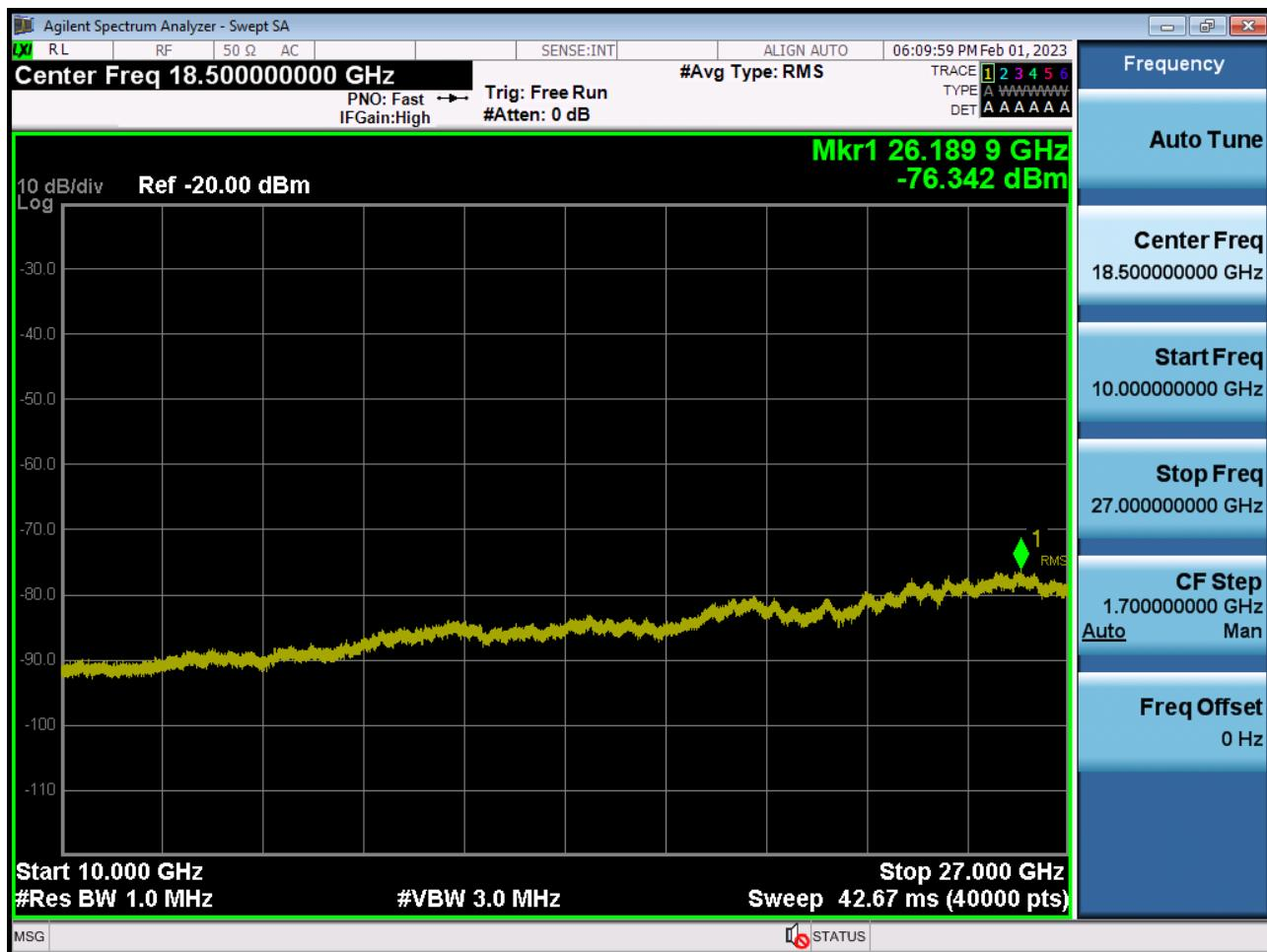
Conducted Spurious Plot 1 (10 MHz Ch.39700 QPSK RB 1, Offset 0)
