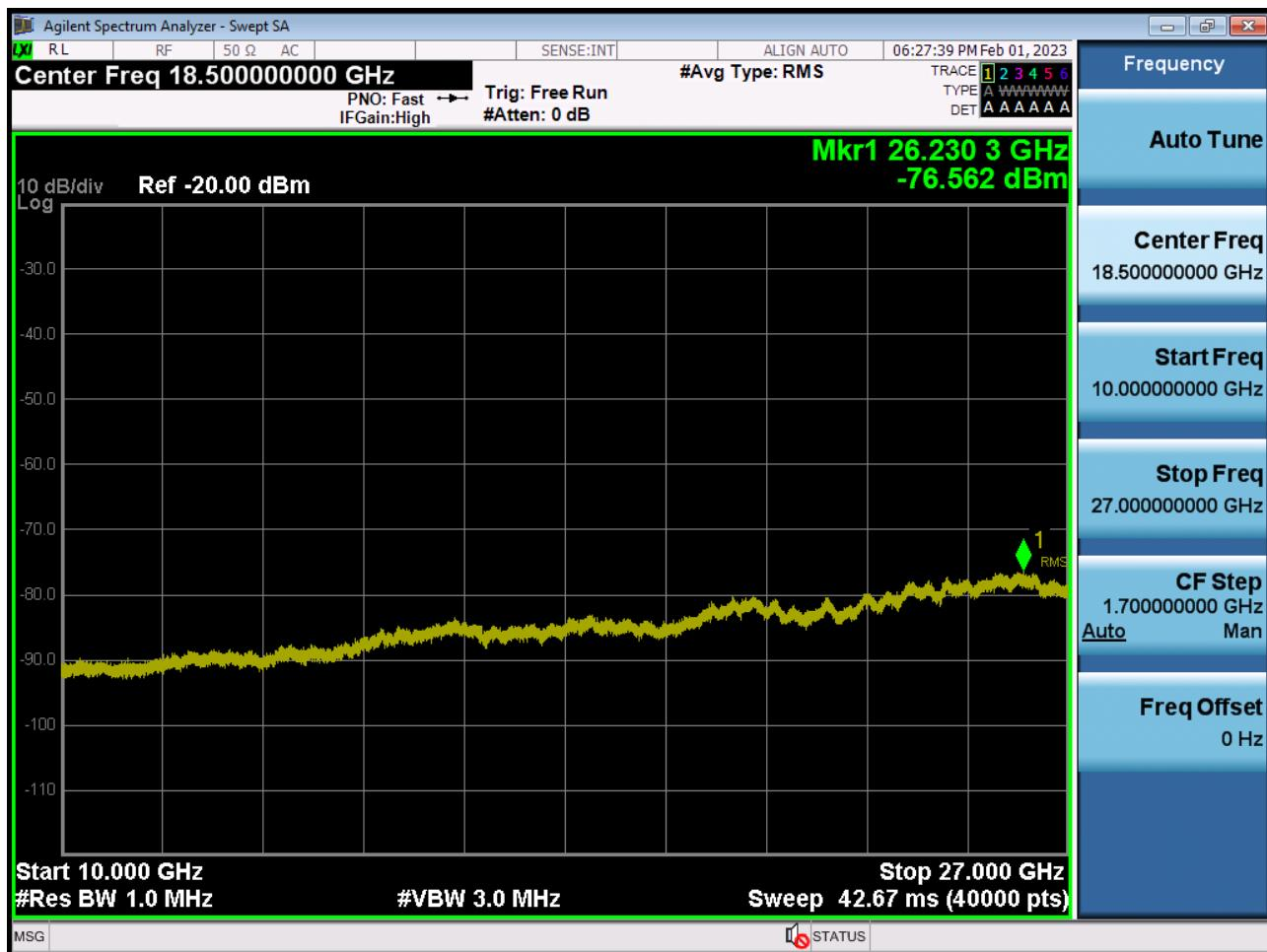
Conducted Spurious Plot 1 (15 MHz Ch.41515 QPSK RB 1, Offset 0)
