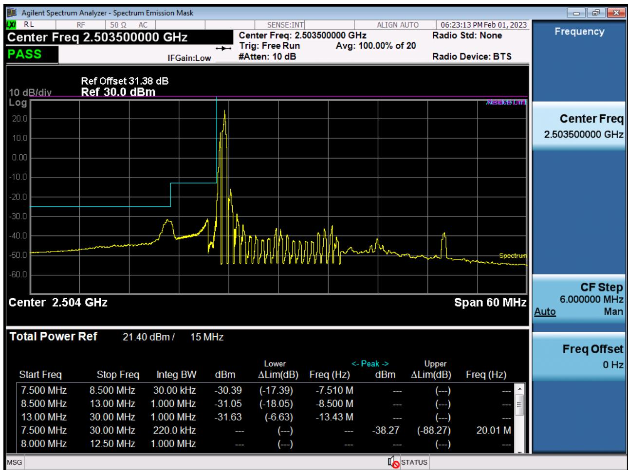
Low Channel Edge Plot (15 MHz Ch.39725 QPSK RB 1, Offset 0)-2
