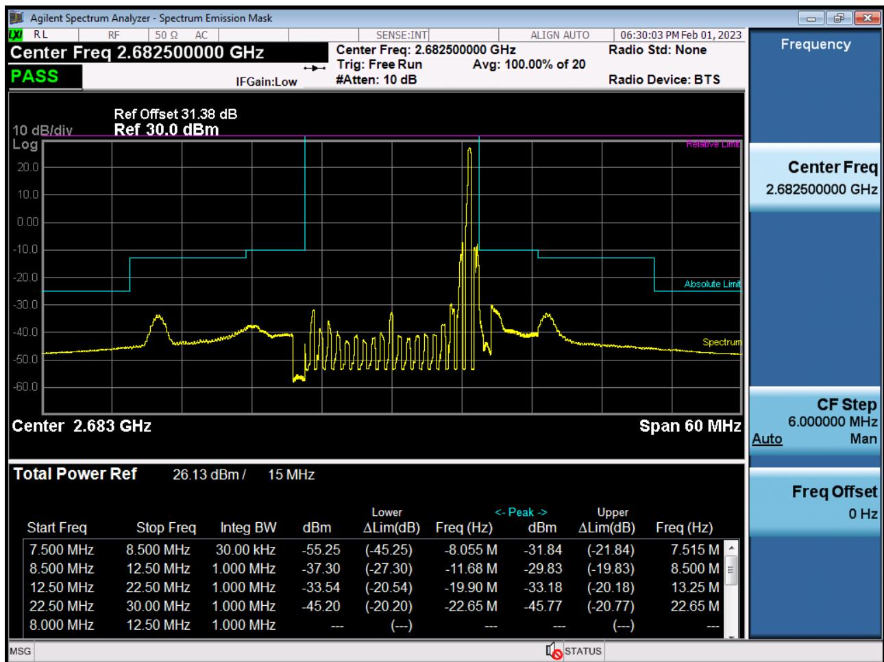
High Channel Edge Plot (15 MHz Ch.41515 QPSK\_RB75\_Offset 0)
