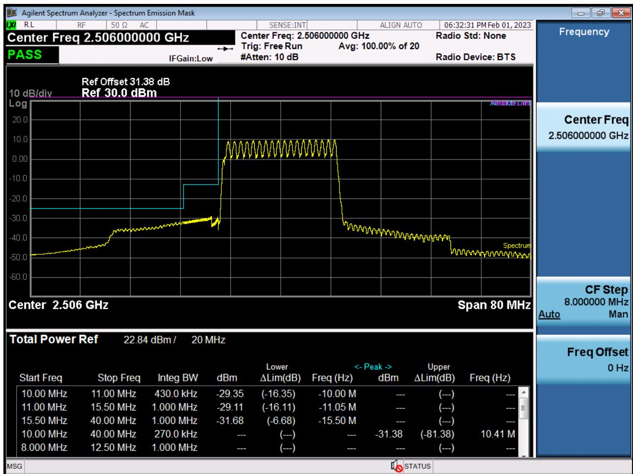
Low Channel Edge Plot (20 MHz Ch.39750 QPSK\_RB100\_Offset 0)-1
