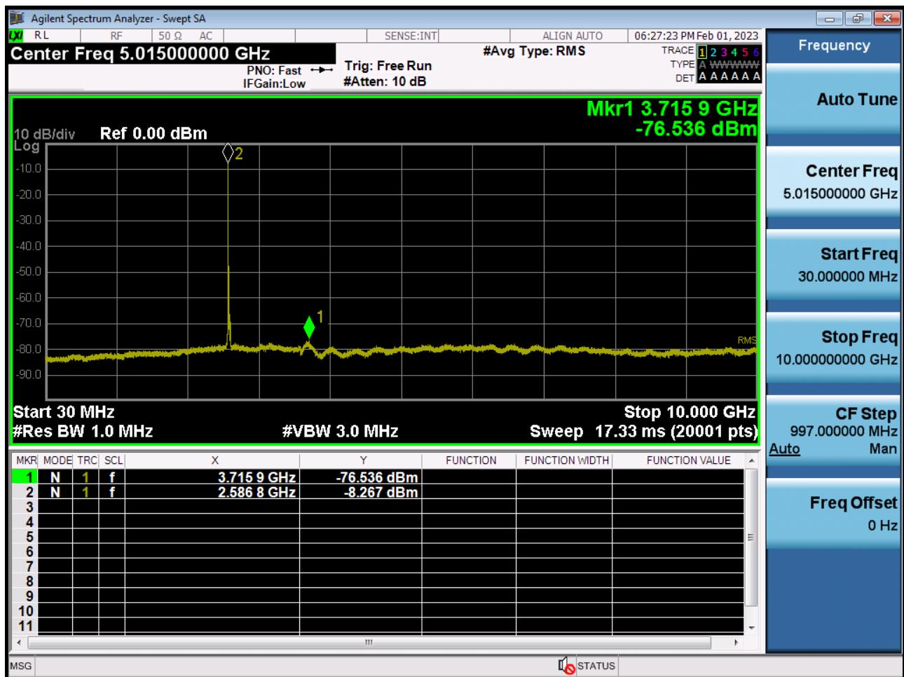
Conducted Spurious Plot 2 (15 MHz Ch. 40620 QPSK RB 1, Offset 0)
