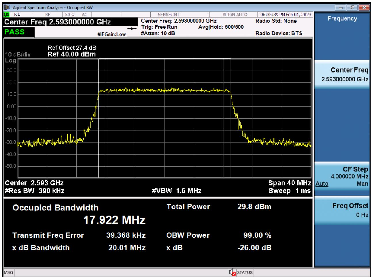
Occupied Bandwidth Plot (20 MHz Ch.40620 64-QAM RB 100)
