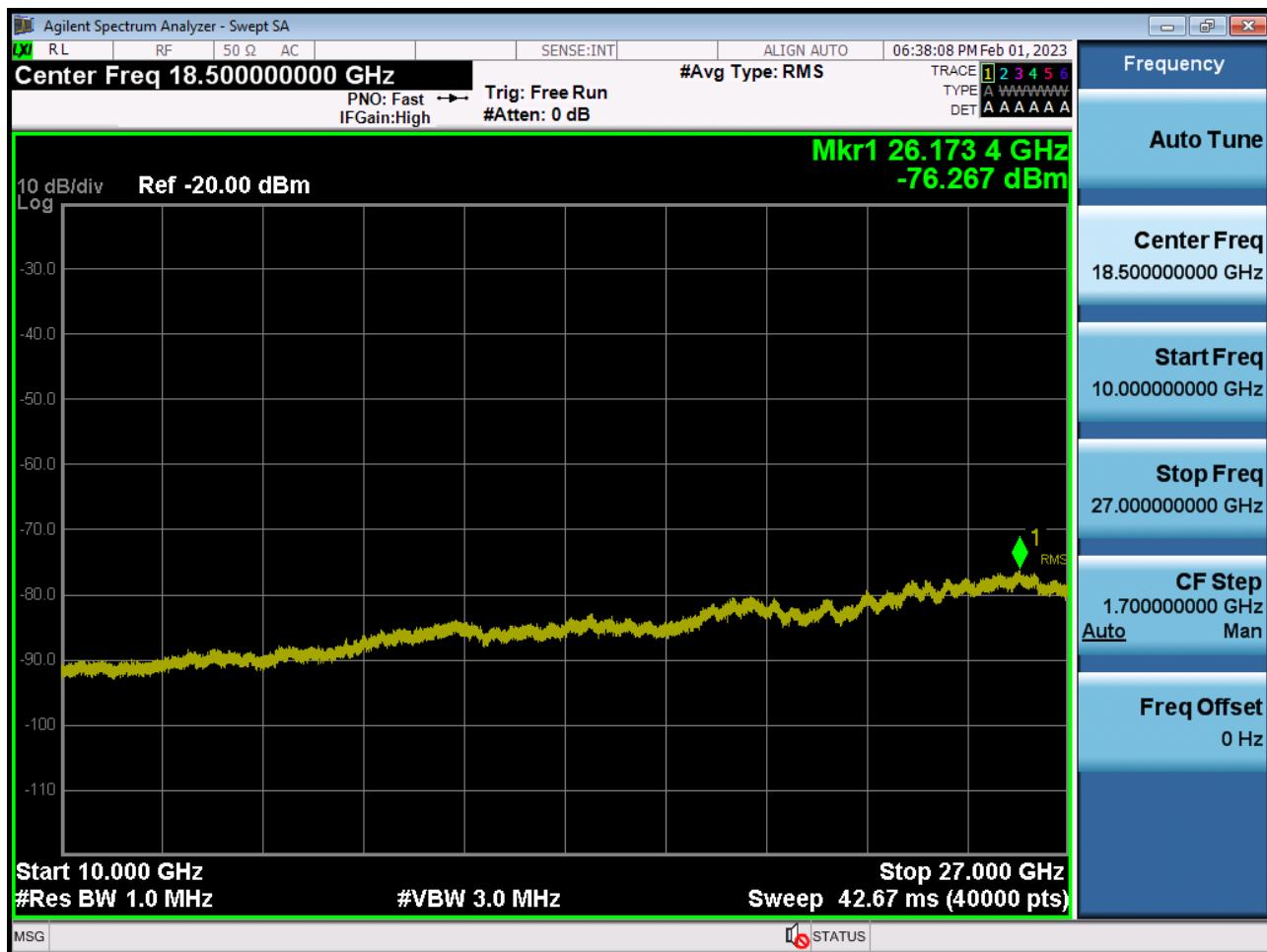
Conducted Spurious Plot 1 (20 MHz Ch.41490 QPSK RB 1, Offset 0)
