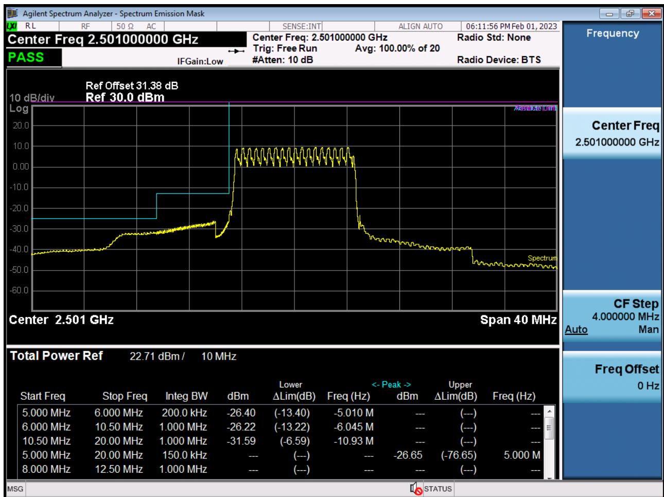
Low Channel Edge Plot (10 MHz Ch.39700 QPSK\_RB50\_Offset 0)-1
