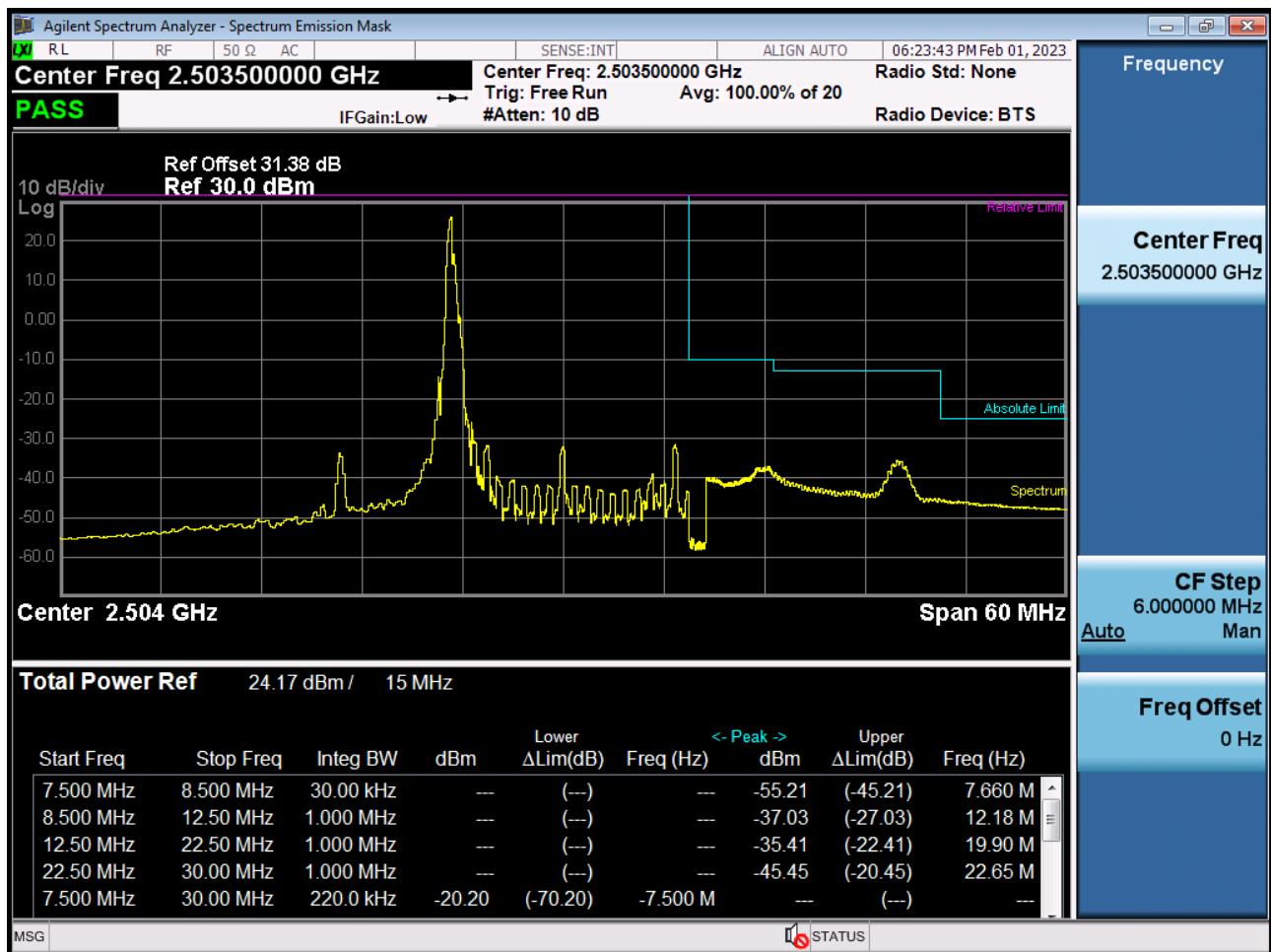
Low Channel Edge Plot (15 MHz Ch.39725 QPSK\_RB75\_Offset 0)-2
