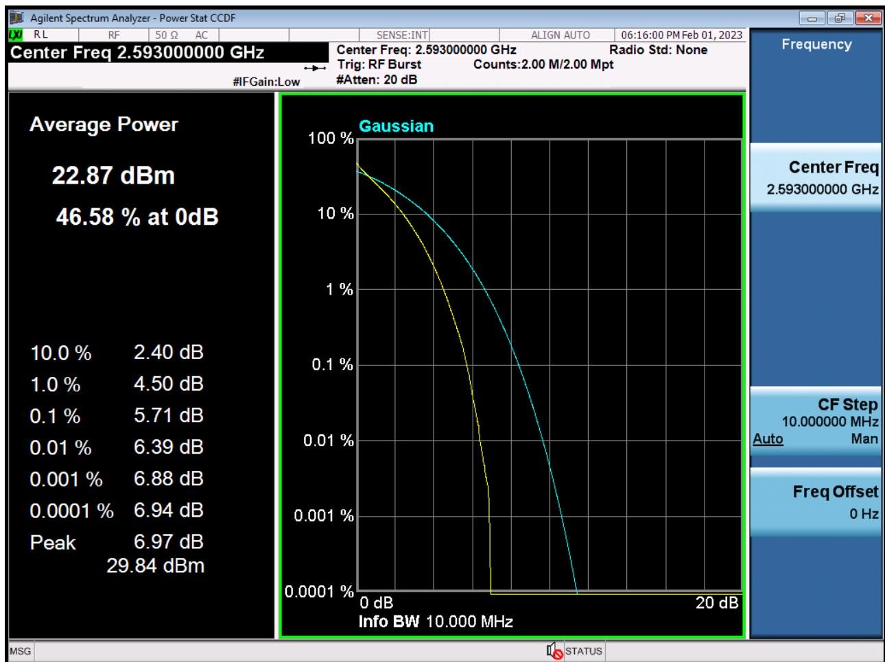
PAR Plot (10 M BW\_Ch.40620\_16QAM\_RB50\_0)
