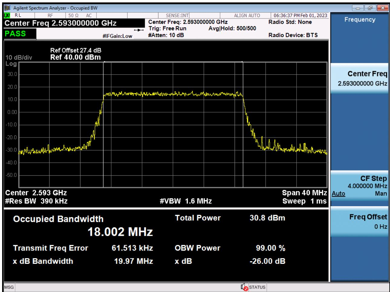
Occupied Bandwidth Plot (20 MHz Ch.40620 16-QAM RB 100)
