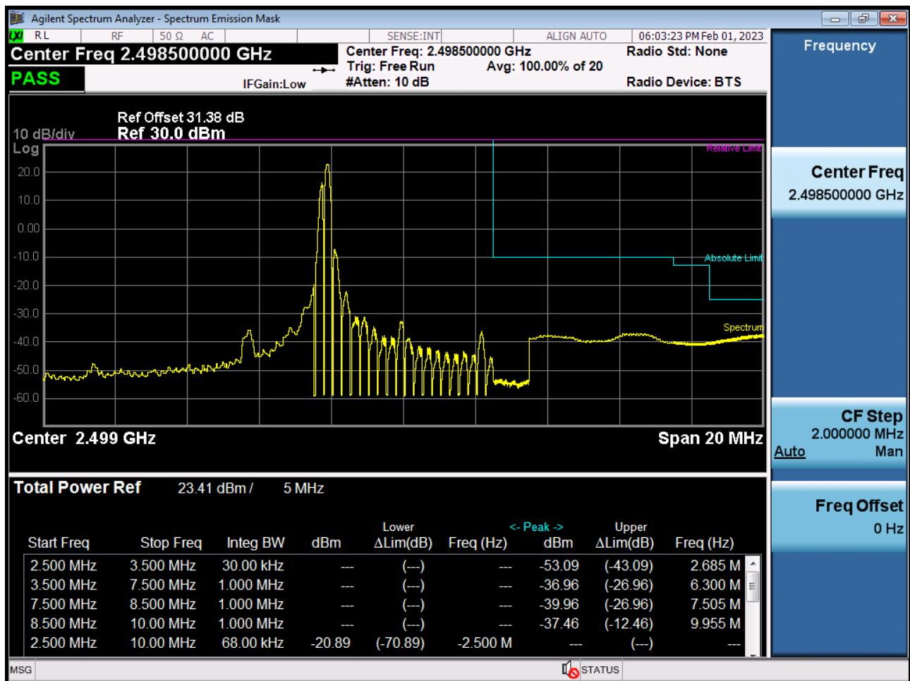
Low Channel Edge Plot (5 MHz Ch.39675 QPSK\_RB25\_Offset 0)-2
