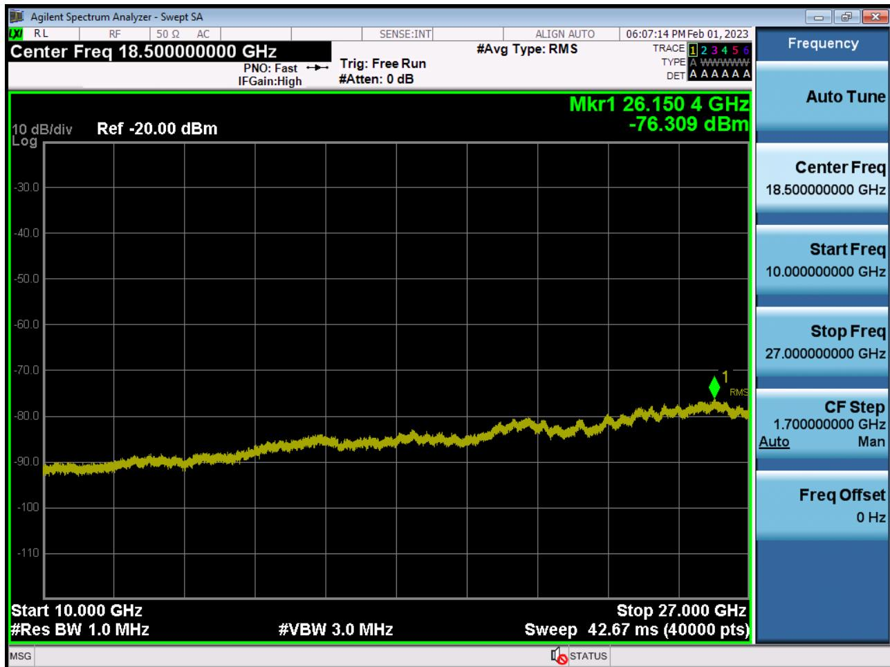
Conducted Spurious Plot 1 (5 MHz Ch.41565 QPSK RB 1, Offset 0)
