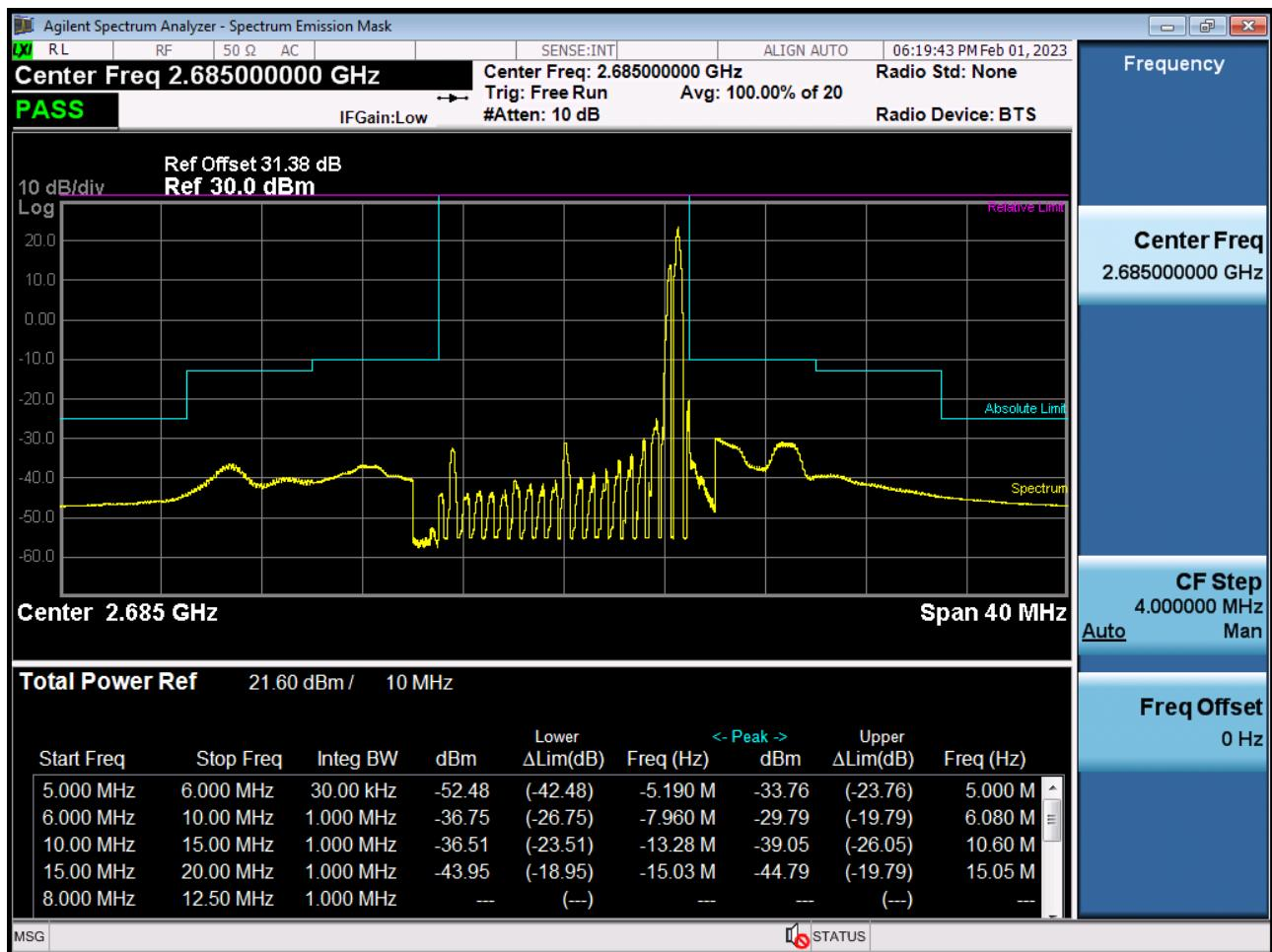
High Channel Edge Plot (10 MHz Ch.41540 QPSK\_RB50\_Offset 0)
