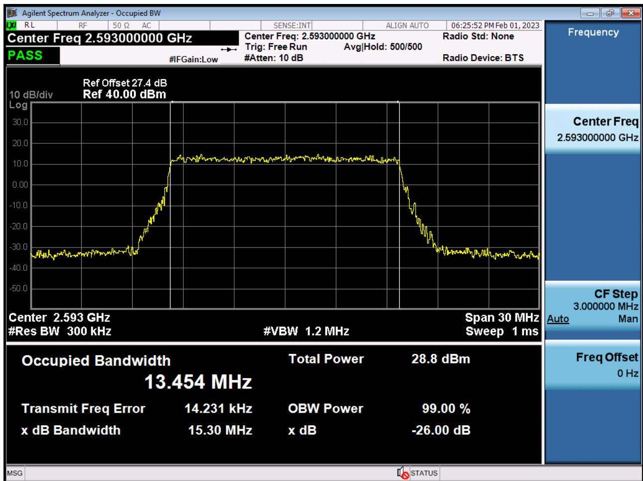
Occupied Bandwidth Plot (20 MHz Ch.40620 QPSK RB 100)
