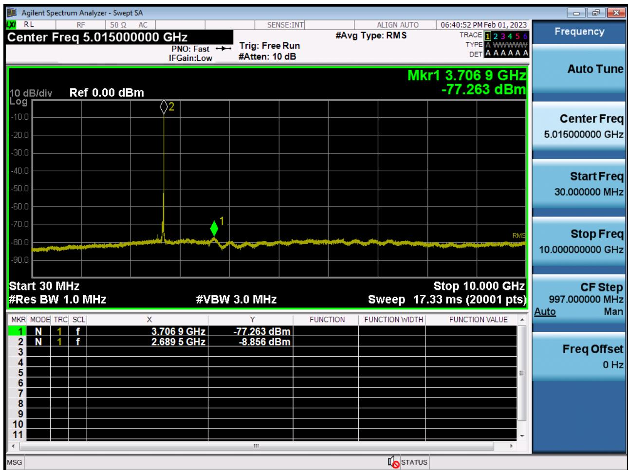
Conducted Spurious Plot 2 (20 MHz Ch. 41490 QPSK RB 1, Offset 0)
