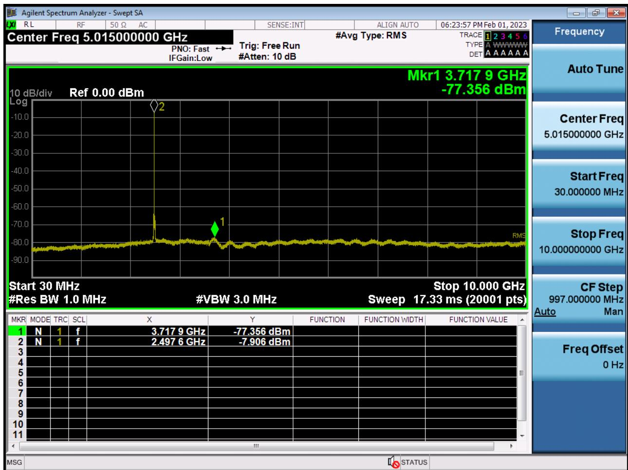
Conducted Spurious Plot 2 (15 MHz Ch. 39725 QPSK RB 1, Offset 0)
