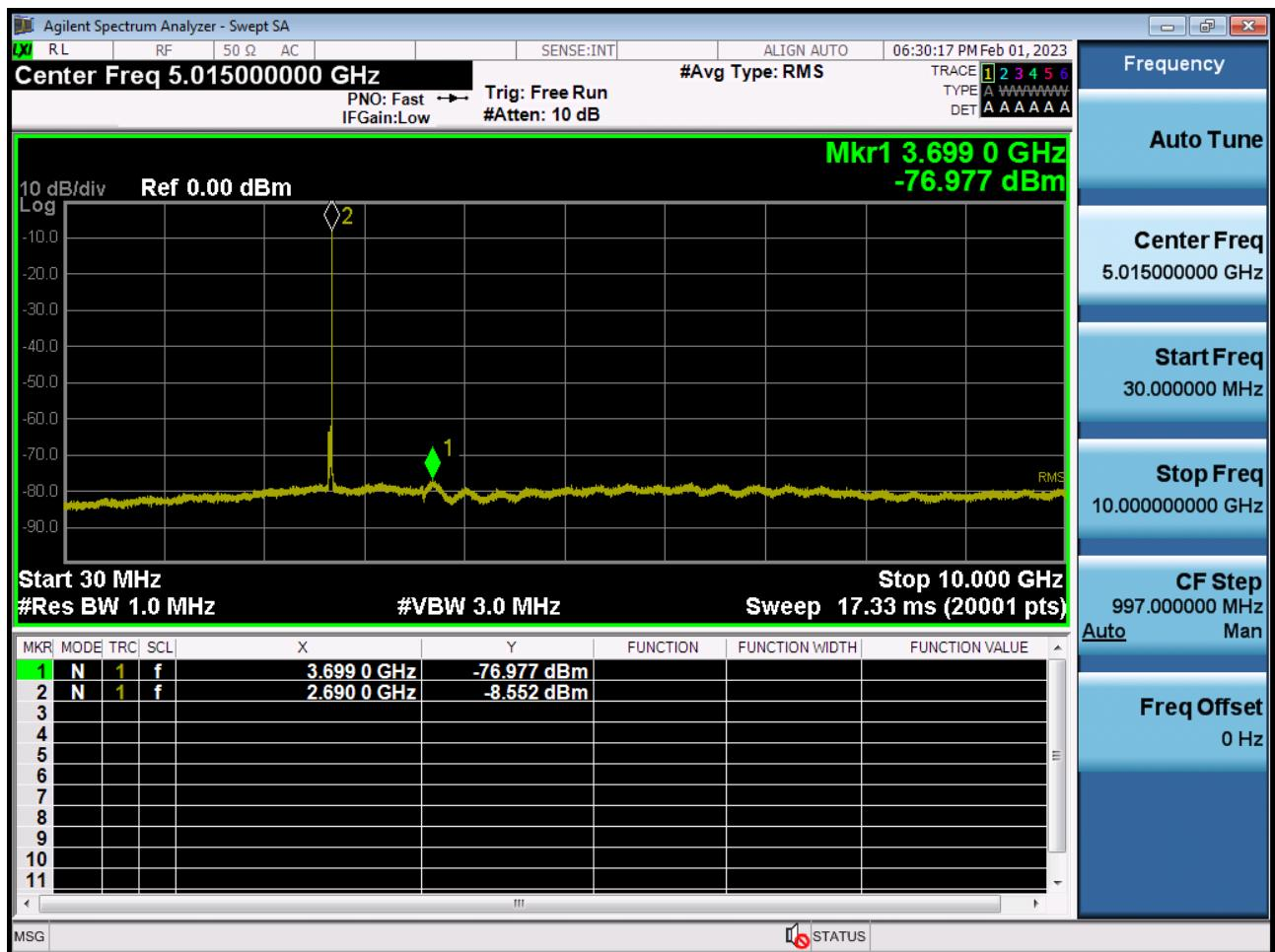
Conducted Spurious Plot 2 (15 MHz Ch. 41515 QPSK RB 1, Offset 0)
