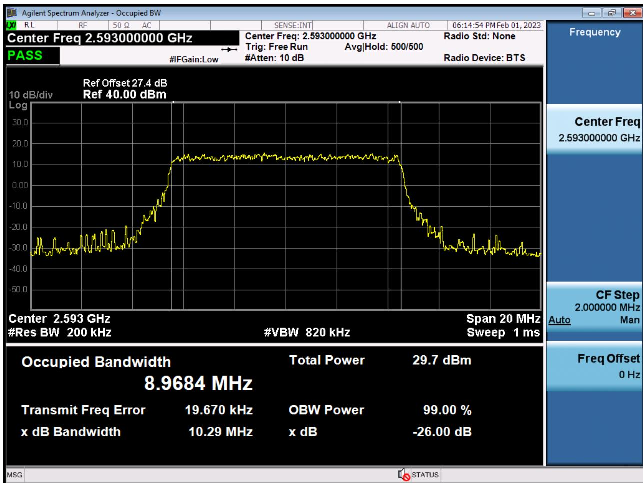
Occupied Bandwidth Plot (10 MHz Ch.40620 64-QAM RB 50)
