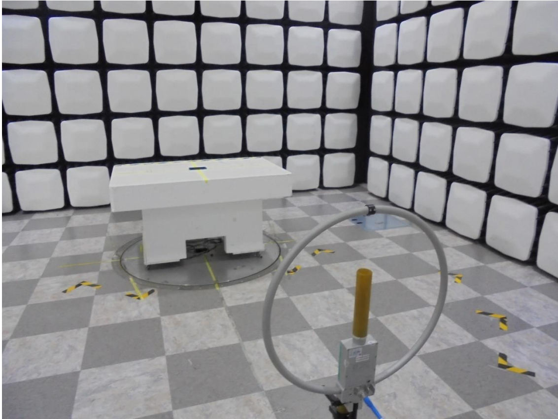
NFC Radiated Test Setup Photo(9 kHz - 30 MHz)
