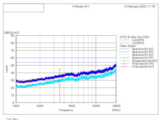
No. Frequency (P) Reading Reading c.f Result Result Limit Limit Margin Regult AV PK AV PK AV RY AV [dB(uV)] [dB
